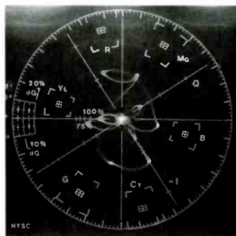
COLOR ACCURACY. The shortfall and counterclockwise rotation of the color vectors in this vectorscope photo indicate low color saturation and some hue distortion.
