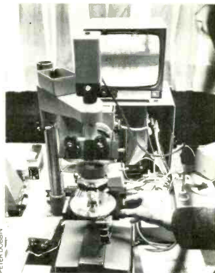
A Compact Disc is examined under a high-power microscope for surface flaws in a Philips laboratory in Holland.
