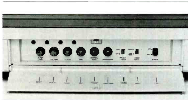
THE MAIN CONTROLS , behind a small door below the screen, include (left to right) BLACK LEVEL (brightness), PICTURE (which adjusts contrast, brightness, and color saturation together), COLOR , TINT , VERTICAL HOLD , and SHARPNESS . A button to the right overrides these adjustments, returning the monitor to its factory settings. The remaining buttons are for input and power switching.
