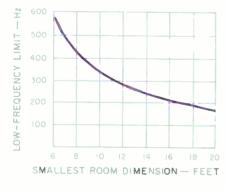
Fig. 4—Lowest effective frequency for acoustic-panel absorbers as a function of room size (where f = 3,390/smallest room dimension in feet). For frequencies below those shown, other forms of absorption (such as wave cavities) would be needed.
