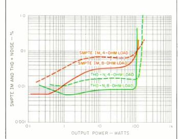
Fig. 7—Distortion vs. frequency, 702 amp, showing THD + N at 1 kHz, and SMPTE IM, for 8- and 4-ohm loads.
