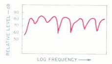
Fig. 2—Frequency response of reference loudspeaker system under anechoic conditions (A) and with effects of early reflections (about 1.1 mS delay) added (B). (After Davis.)
