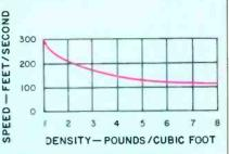
Fig. B1—Speed of sound versus packing density of material. Speed in air is normally 1,130 feet per second. (After Bradbury.)
