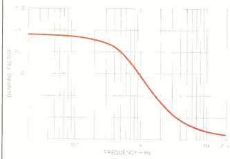
Fig. 10—Damping factor vs. frequency, right channel, 702 amp.
