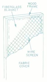
Fig. 3—Photo and cutaway view of absorption panel's construction. The panel should have a solid backing (not shown).
