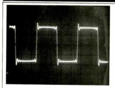
Fig. 6—Reproduction of a 1-kHz square wave.
