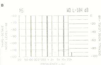
Fig. 2—S/N analysis, both unweighted (A) and A-weighted (B).
