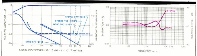
Fig. 1—Mono and stereo quieting and distortion characteristics, FM section.
