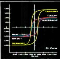
Comparison of the magnetic flux of Triad EM-X vs. two leading tapes under identical recording conditions. EM-X records approximately twice the signal, for increased dynamic range and lower distortion at higher signal levels.
