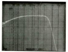
Fig. 5—Frequency response, AM section.
