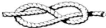
FIGURE OF EIGHT KNOT — As for an overhand knot, but easier to undo.
