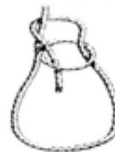
TIMBER AND HALF HITCH — Useful for hoisting lengths of timber. Only safe when additional half hitch is put on end of hauling part.
