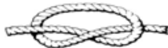
OVERHAND KNOT — To make a stop on a rope, to prevent the ends from fraying or to prevent it slipping through a block.
