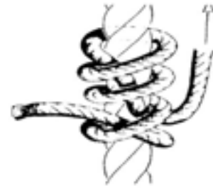
ROLLING HITCH — To secure stopper, or two ropes pulling in opposite directions. Very useful, preferable to clove hitch or blackwall hitch, providing rolling turns are put on in proper direction of pull. Safe.
