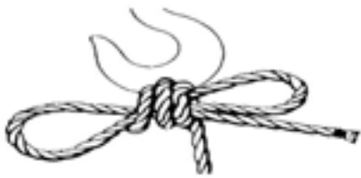
(i) Single Snotter Shortener partly made. Two bights ready to be placed on hook.
