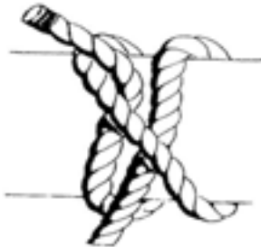
CLOVE HITCH — Used to commence rope lashings. Not safe for other purposes unless ends secured, with additional half-hitches.
