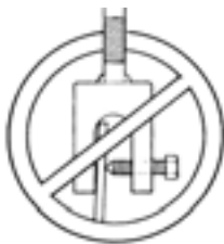
Do not use home made type plate clamps or plate dogs.
