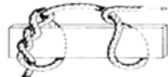
TIMBER AND HALF HITCH — Useful for hoisting lengths of timber. Only safe when additional half hitch is put on end of hauling part.
