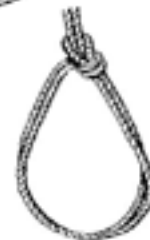
(c) BOWLINE ON THE BIGHT . The bowline on the bight is formed by making the first part of a bowline with the bight of the rope and passing the whole hitch through its bight.
