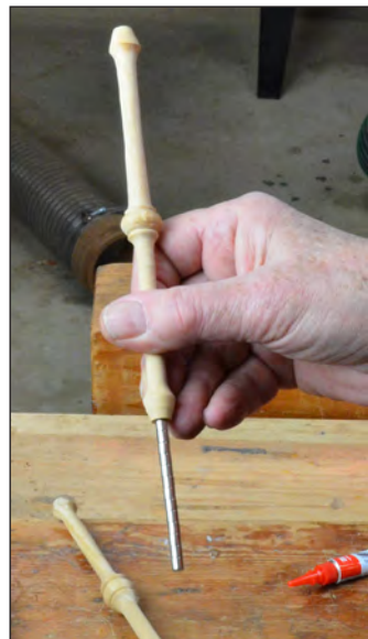
17. Manage — Stick the stack to the installed magnet and turn the rod end for end so the empty hole is at the top. Put a drop of CA glue in the hole.
