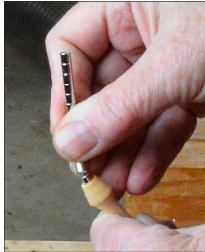
15. Magnet — Insert one end of the magnet stack into the bored hole. Swipe sideways to separate, don't pull.
