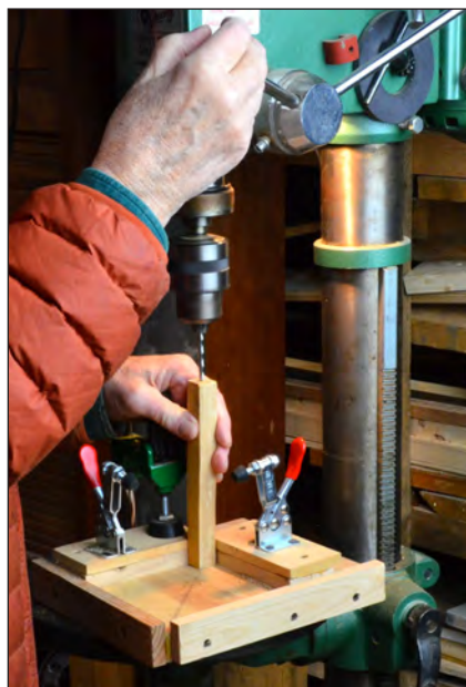
6. Boring — Stand the rod on end to bore for cylindrical magnets; the shopmade fixture centers it. Bore the exact length of the magnet plus a smidge.
