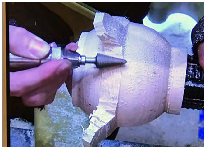
Oudet power-carves most of the collar away, leaving just enough wood for the spout. He uses the lathe to hold the workpiece.
