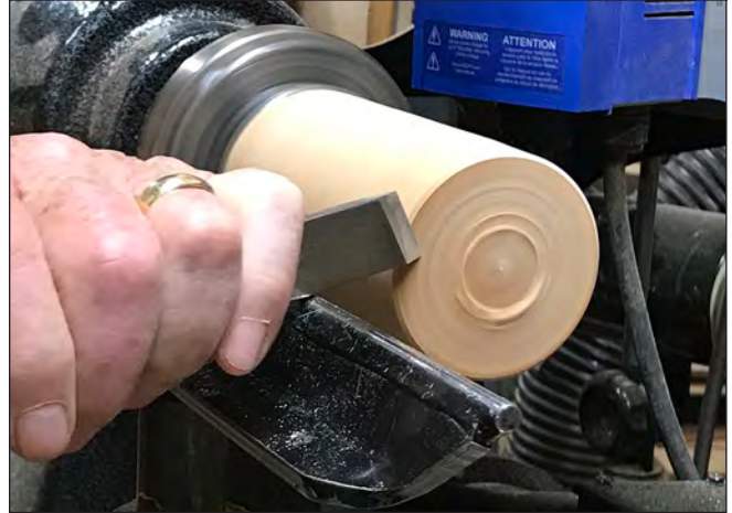
4 — Skew pares end of glue block. It needs to be flat and smooth.
