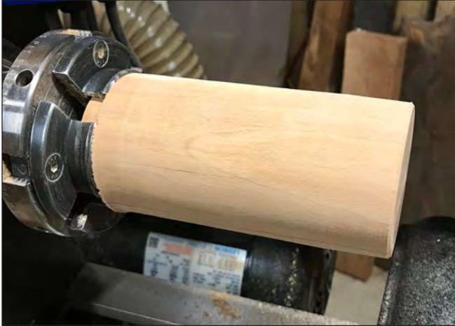
3 — Tenon the glue block, mount it in the scroll chuck, and turn a clean cylinder.
