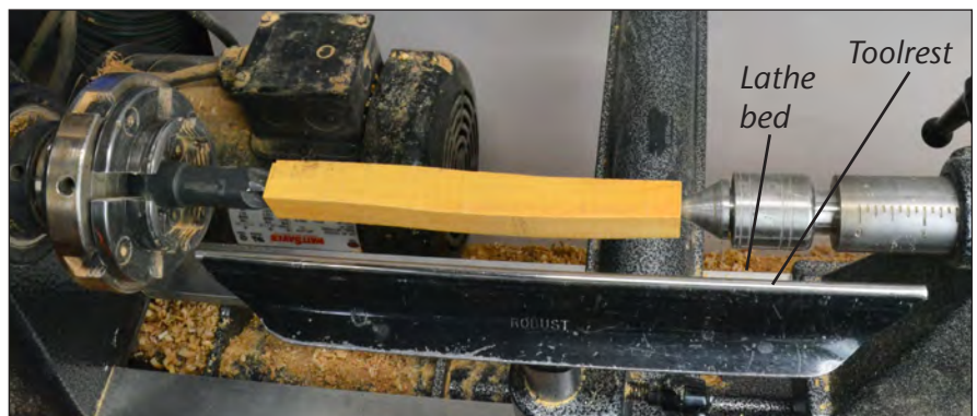
7. Centering — A small, spring-loaded four-prong drive center is perfect for this job.
