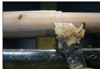
(Right) Peel cut the cylinder to 3/4" (19mm) diameter, stepping down the length of the blank.
