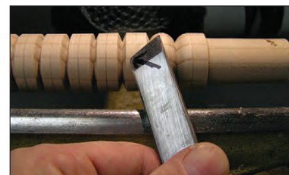
Roll beads with the goal of leaving the marked centerline at their peak. End with the skew's cutting edge vertical.
