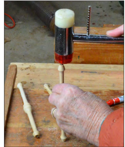
16. Mallet — Tap the magnet flush using a non-ferrous mallet on a wooden bench. Note the magnet stack parked on the mallet shaft.
