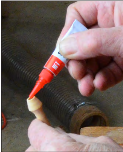
14. Glue — A drop of cyanoacrylate glue in the bored hole will secure the magnet.
