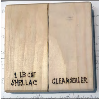
Carol passed around samples of poplar sealed two ways, labeled with a pen burner.
