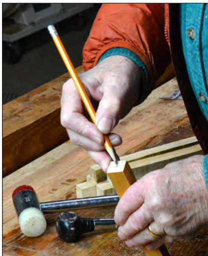
5. Marking — Eyeball the center of the blank, mark it, and make a dimple with an awl or centerpunch.
