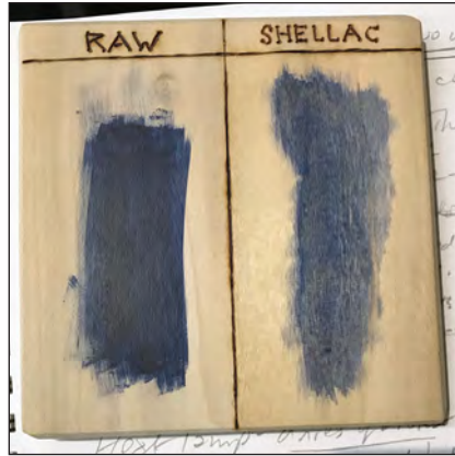
Carol's sample shows paint on raw wood is opaque, left; paint over shellac, right, is translucent and the grain shows through.
