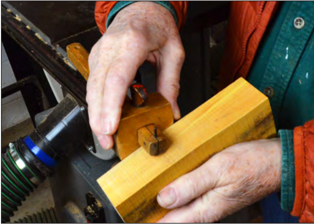
3. Layout — The marking gauge, set to 3/4" (2cm), lays out blanks on bandsawn and crosscut-to-length billet of air-dried Bradford pear.
