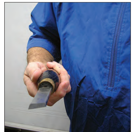
To form the left side of the bead, the hand starts horizontal, then rotates counterclockwise as if to shake at vertical. ↩
