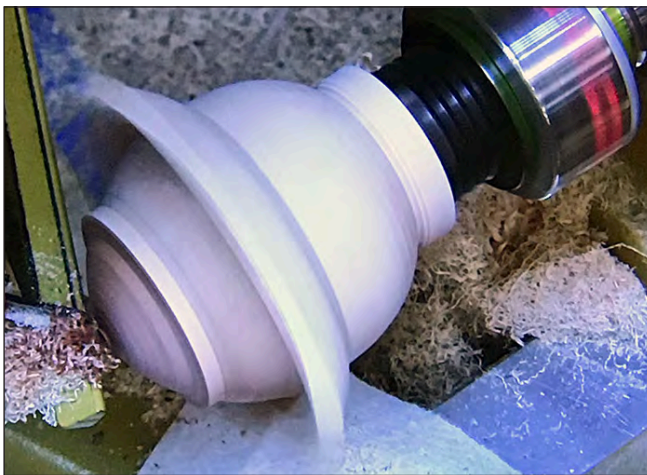
To create a teapot, the turner first makes its body with a broad collar or flange. Then hollow the body before shaping the spout.
