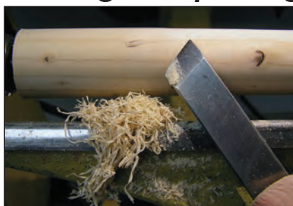
(Left) Plane a cylinder smooth with the skew five to ten times.
