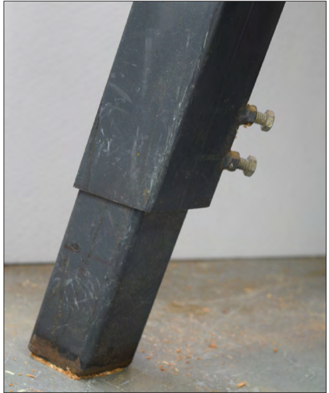
1 - Adjust legs, or use shims, to make sure your stand sits solidly on the floor.
