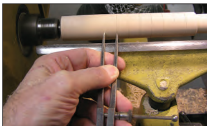
Plane a cylinder smooth with the skew, and mark out 5/8" (16mm) intervals.
