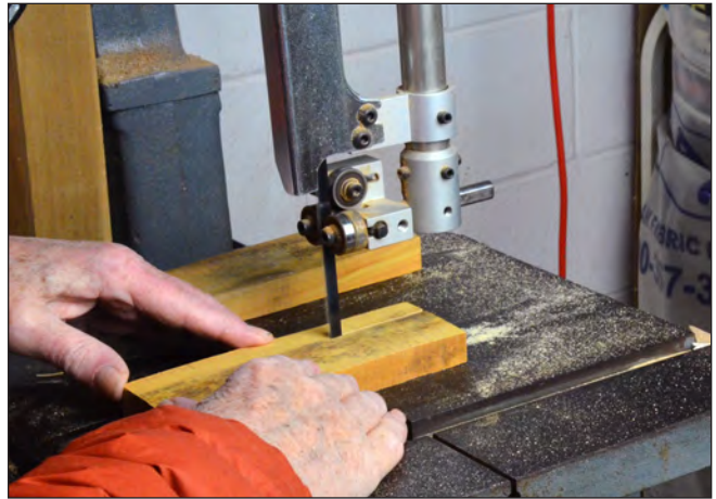
4. Bandsaw — Push and guide the blank by its sides and corners, so your hands never cross the blade's path.
