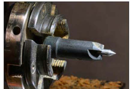
7. Centering — A small, spring-loaded four-prong drive center is perfect for this job.
