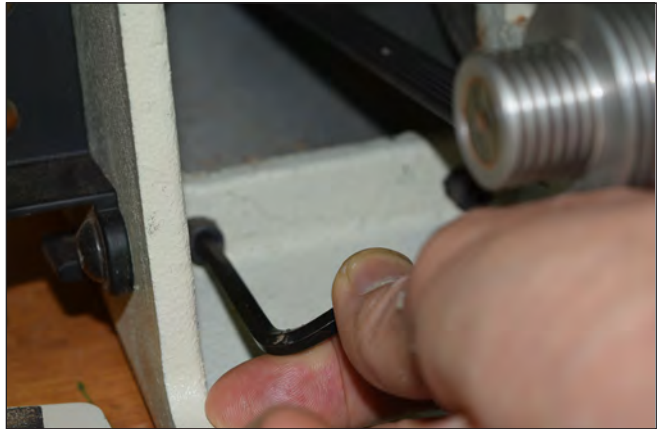
4 - Check that all bolts connecting the headstock to the lathe ways are tight.
