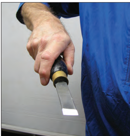
Bead rolling. To form the right side of a bead, the turner's hand rotates clockwise...
