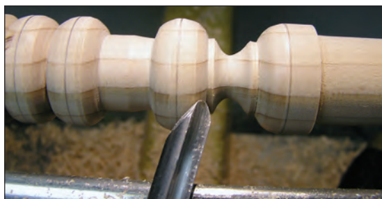
Plane a cylinder smooth with the skew, and mark out 5/8" (16mm) intervals. Form V-grooves at every mark about 1/4" (6mm) deep, then mark centerlines between all the V-grooves. Roll beads as above, then
