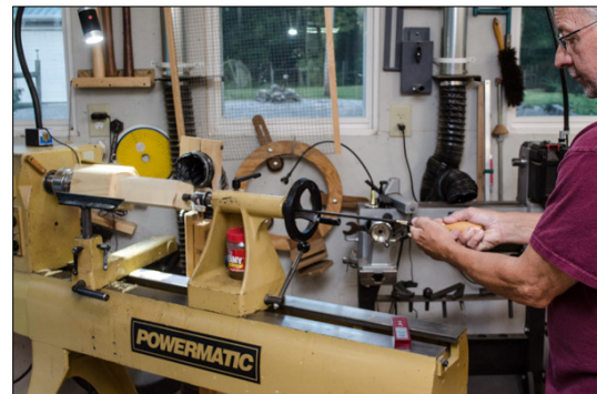
Boring with lamp auger
