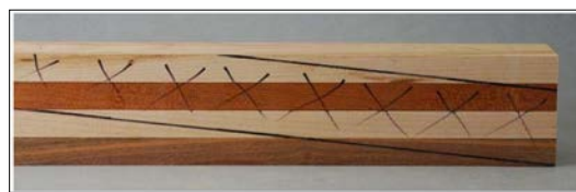
Figure 3 - Mark-out the Glued-Up Blanks
