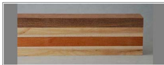
Figure 2 - Stacked Boards Prior to Glue-Up
