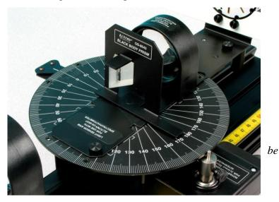
Figure 4: The prism apex should oriented toward the light source.
