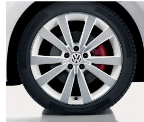
19 inch 'Tornado White' alloy wheels with 235/40 R19 tyres and anti-theft wheel bolts. Image shown is Beetle Sport 2.0 litre TSI 220 PS.
