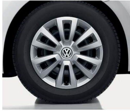
16 inch steel wheels with 215/60 R16 tyres and full size wheel trims.
