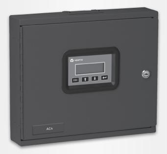
The Liebert AC4 coordinates control of systems with redundant equipment, such as multiple thermal-management units or pumps. The AC4 can control stand-by functions and unit rotation, perform testing on stand-by devices, stage operation based on sensor-reading levels, and monitor alarm status of connected devices. The Liebert AC4 interfaces with any device that closes an electrical contact.
