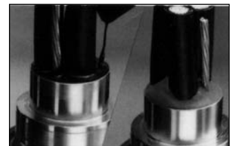
4. Pot cable (using liquid or putty)
