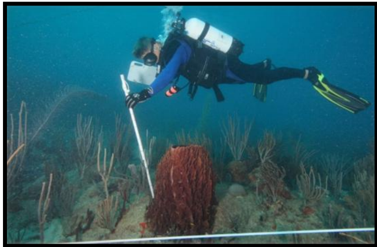
Figure 5-1: Marine sponge assessments allow important ecological and economic services to be evaluated by measuring surface area.
