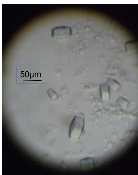
Figure 6.12 Crystals growing in 50 mM phosphate/ citrate, pH4.2, and 26% PEG400 at 4 °C by the hanging-drop vapour-diffusion method.
