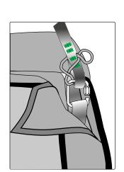
4. 4. Repeat procedures 1,2,3 with an additional O ring for the connection to the harness. Tighten the Maillon Rapide® locking gate securely, with pliers if necessarily.
