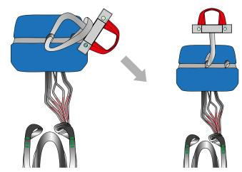
2. Push the handle through the central loopstrap, and make a « loop to loop » connection with the handle.
