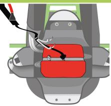
1. Place the risers « J » under flap « A ». Push them through between flap « B » and the upper flap in order to stow away the riser and lines excess from the reserve « K » to the bottom of the pocket.
