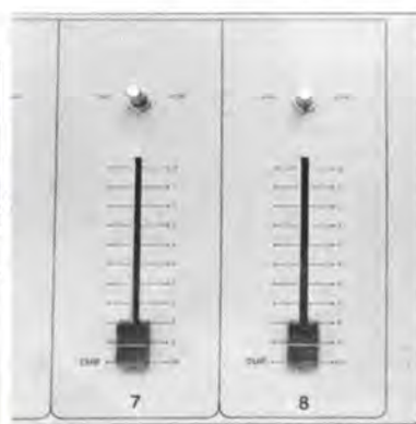
Slide attenuators, rotarys also available
