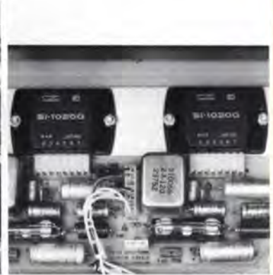
15 watt per channel monitor amplifier
