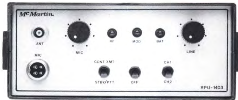
Control panel (top view) of RPU-1403
