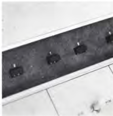
Pushbutton input select switches
