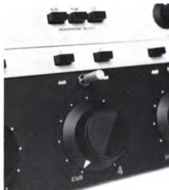
Attenuator, input and program audition select switches
