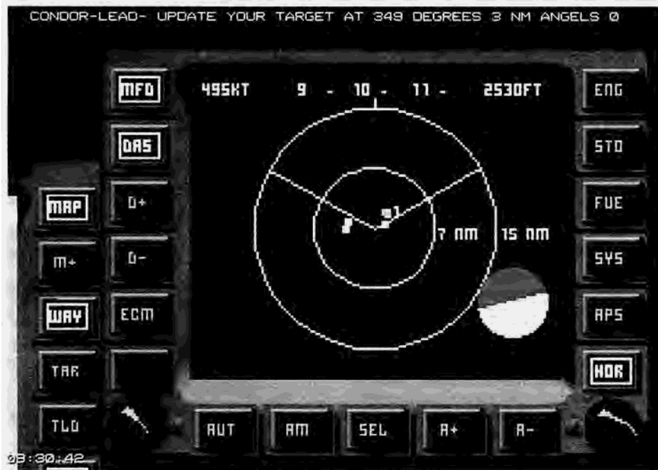
DASS helps automate the job of defending the aircraft
