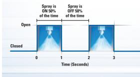
Modular Spray System provides easy control of nozzles and cycle times up to 10,000 cycles per minute.
