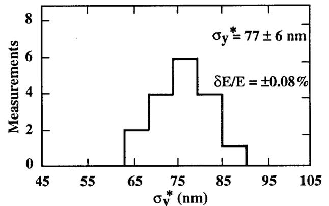
Fig.1 Histogram of spot size measurements. These are raw data, and when corrected the mean is  $\sigma_y = 70$  nm.<sup>6</sup>
