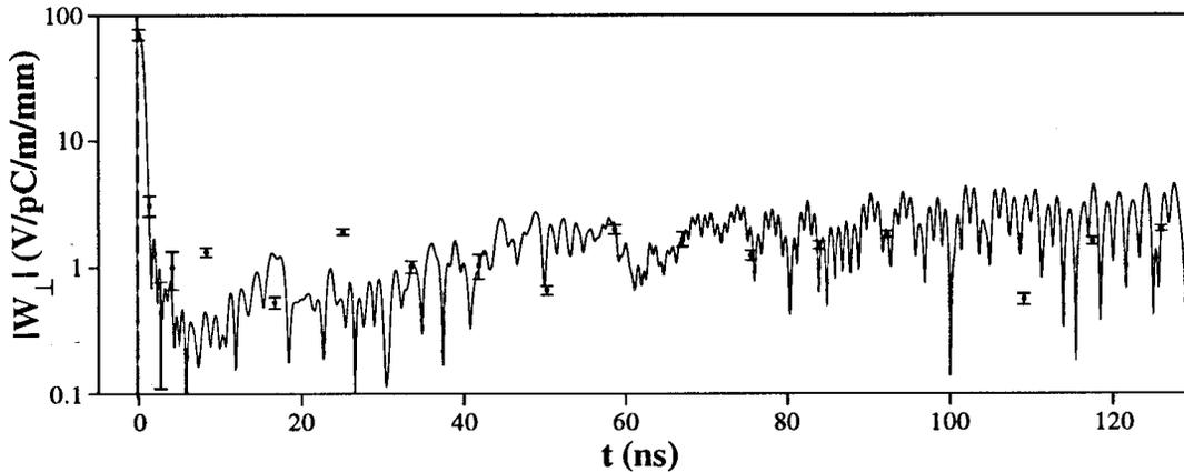
Fig. 2 The amplitude of the dipole wakefield given by the data points is compared with a prediction that assumes that the cells had an rms fractional frequency error of  $1.5 \times 10^{-4}$  in addition to the design frequency spread.<sup>8</sup>
