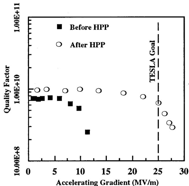
Fig. 3 Results of high power pulsed processing (HPP) of a 5 cell, 1.3 GHz superconducting cavity. Processing was performed with a peak field of 90 MV/m.<sup>18</sup>
