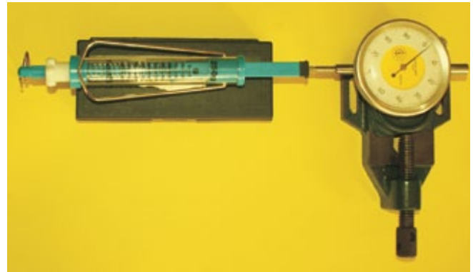
Fig.5. Push/pull spring balance testing resistance force of an analogue dial gage tip.
