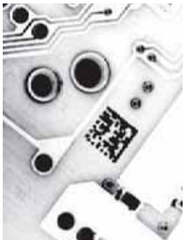
Figure 22 - Data Matrix Code Directly Marked on PCB Surface by Using Laser Etching Technology
