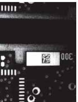
Figure 21 - Dot Matrix Code Directly Marked on PCB Copper Pad by Using Ink-Jet Technology
