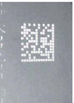
Figure 19 - Dot Peening Marking on Metal Surface with Multi-dot per Code Element
