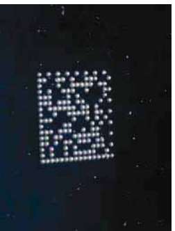
Figure 20 - Directly Marked Dot Matrix Code Characterized by Outstanding Separation Distance between Adjacent Code Elements
