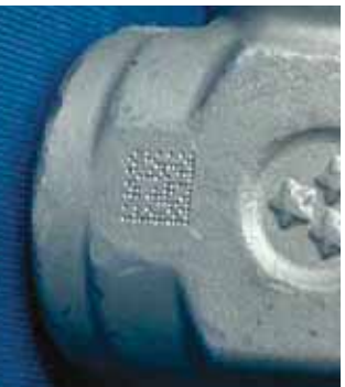
Figure 18 - Dot Matrix Code Directly Marked on Metal Surface by Using Dot Peening Technology
