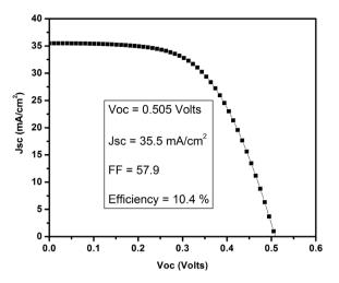
Figure 2. The 1  $\mu$ m Al metal grid pattern based CIGS solar cell current-voltage (I-V) output photo conversion efficiency curve.
