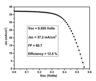
**Figure 4.** The 200 nm Al/800nm Cu metal sandwich grid pattern based CIGS solar cell current-voltage (I-V) measurement output and photo conversion efficiency curve.
