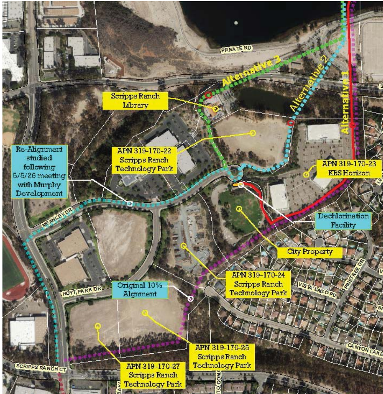
Figure 3: Pure Water Pipeline Re-alignment to eliminate easements
