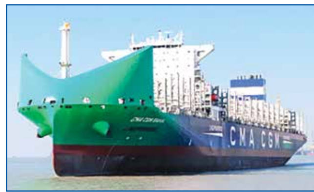
CMA CGM is adding a larger wind deflector or "bowshield" to improve fuel efficiency.
