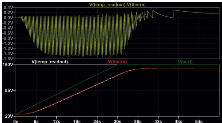
Figure 2: The direct transient circuit simulation shows the temperature profile of the application. Top: External temperature V_{\text{surf}} , thermistor temperature V_{\text{therm}} and digitized measured value ( t_{\text{on}} = 200 \text{ ms} , n = 10 ). In the bottom window: Difference between measured value and actual thermistor temperature
