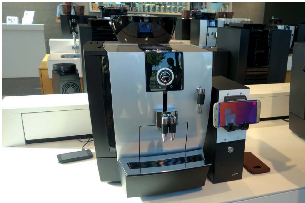
Functional demonstrator with a standard coffee machine, a scoop terminal with Secure Element, and a conventional "insecure" smartphone as the e-money source.
