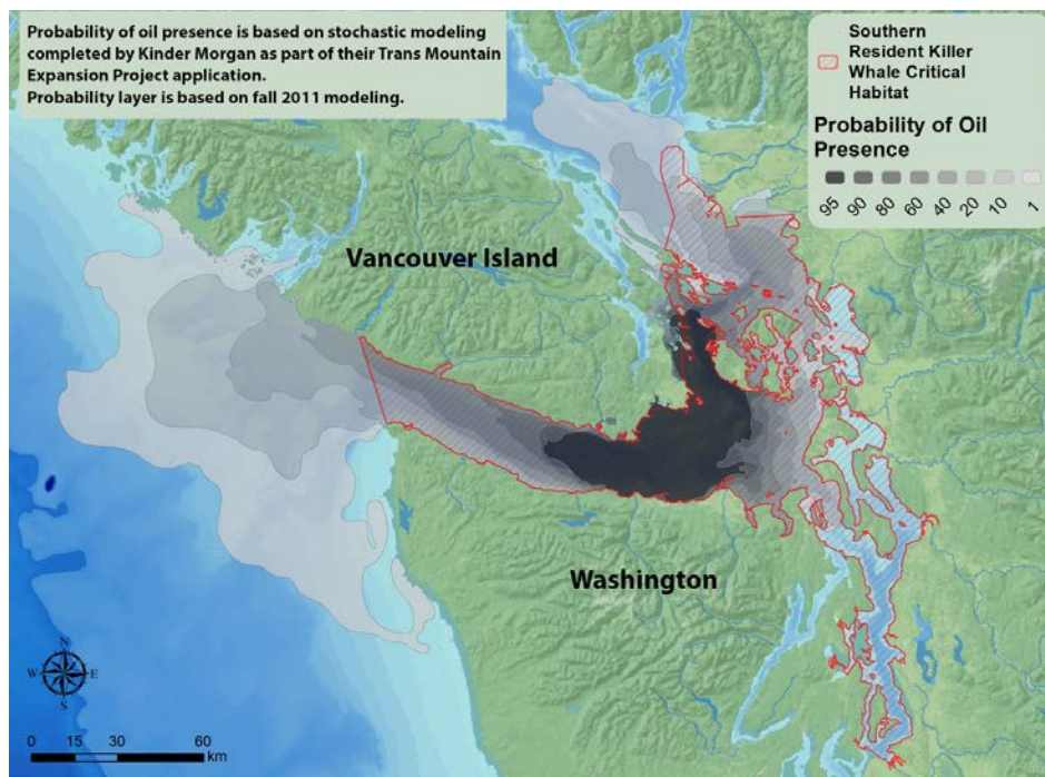
Figure 1.1 Black to grey shading indicates the probability of oil presence 15 days following a 15,000 m 3 fall spill of diluted bitumen at Arachne Reef in northern Haro Strait, BC. The modelled probabilities of oil presence (EBA 2013) are overlaid with the Critical Habitat of Southern Resident killer whales in Canada and the United States. Source: AJR et al. 2017
