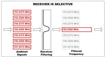
Figure 16: Properly Designed Receiver Filtering of Adjacent Channels
