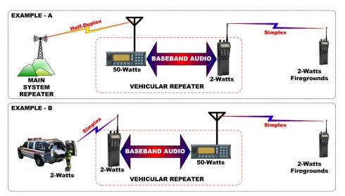
Figure 13: Simple Vehicular Repeater Utilizes Mobile Radio and Handheld Radio
