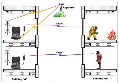
Figure 28: ACU-M Gateway Repeaters Positioned in Adjacent Building
