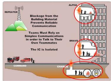
Figure 10: Building Material Blocks Communications Signals to the Outside
