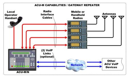
Figure 21: ACU-M Supporting (4) LMR's, (2) VoIP Links & (1) Operator's Handset
