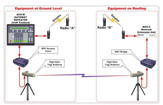
Figure 26: Block Diagram of Extended WiFi Link
