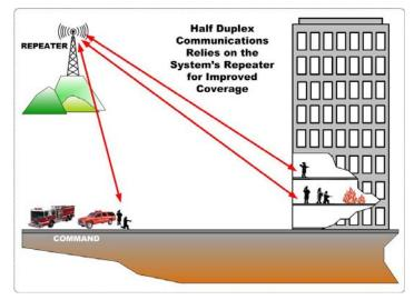
Figure 9: Firegrounds Communications Utilizing the System Repeater
