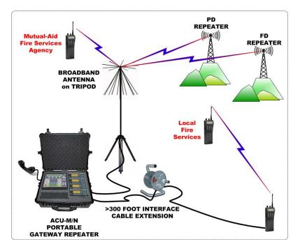
Figure 22: ACU-M Portable Gateway Repeater Mounted in Armored Case
