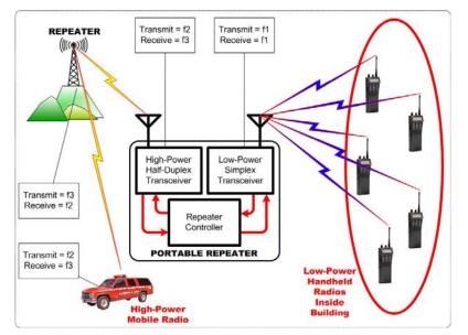
Figure 11: Portable Repeater Rebroadcast Simplex Communications
