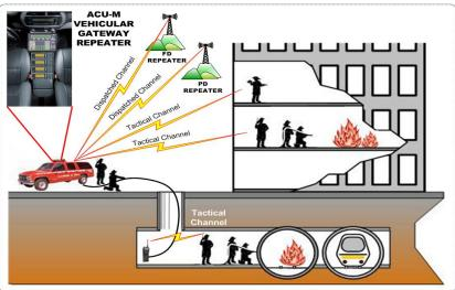
Figure 23: ACU-M Vehicular Gateway Repeater Mounted Battalion Chief's Vehicle
