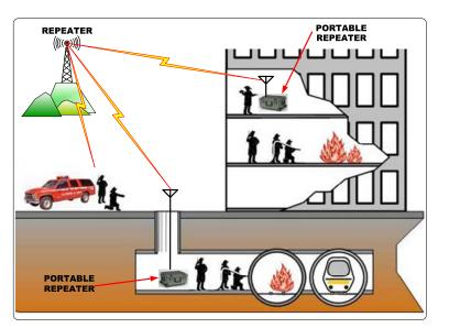
Figure 12: Portable Repeaters Located Inside Building, or Below-Grade
