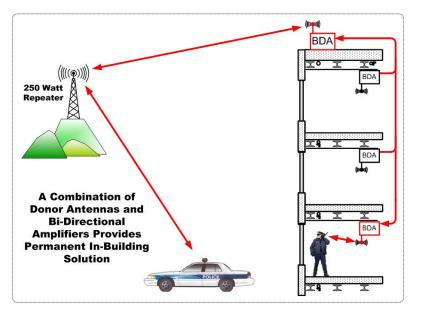
Figure 4: Bi-Directional Amplifiers, Permanent Solution
