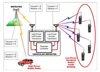
The biggest advantage of a vehicular repeater is that it does not need to be carried into the building; it can remain on the apparatus where power is not an issue (see Figure 14).
