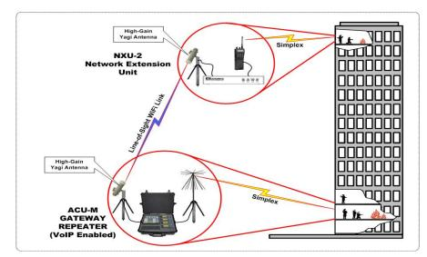
Figure 27: ACU-M Utilizing its Optional VoIP Feature with an Extended WiFi Link
