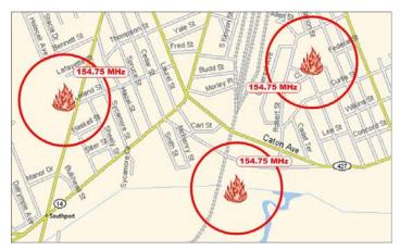
Figure 8: Several Simplex Firegrounds are Reusing the Same Frequency
