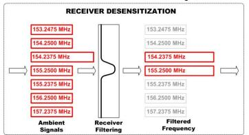
Figure 17: Receiver is "Desensed" From Adjacent High Power Transmitter
