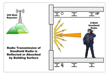
Figure 1: Blockage or Absorption of Low-Power Handheld Radio Transmission
