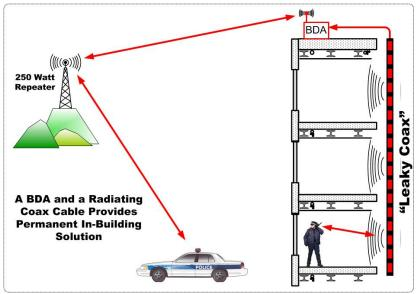
Figure 5: Radiating Cable, Permanent Solution
