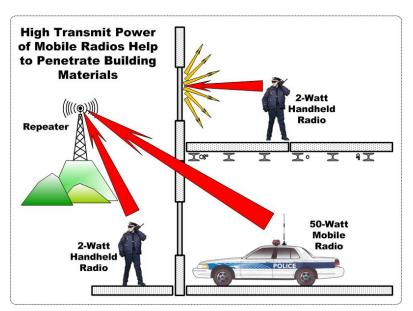
Figure 2: High-Power Mobile is able to Penetrate Building Material
