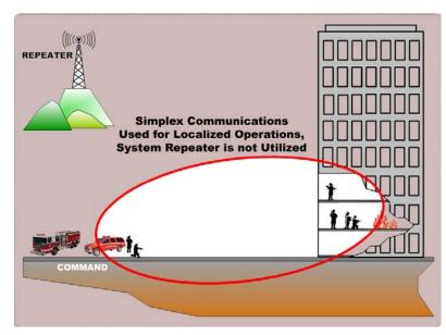
Figure 7: Simplex Firegrounds Communications Does Not Rely on Repeater
