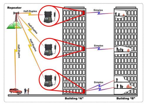
Figure 29: ACU-M Gateway Repeaters Links all Simplex Users through the Repeater
