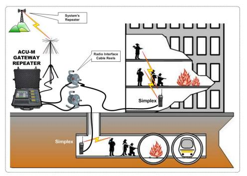
Figure 25: Use of Long Radio Interface Cables
