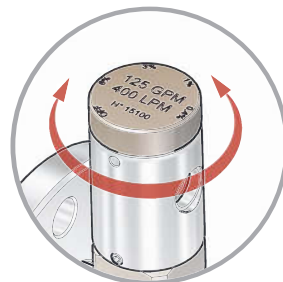
Suction percentage set with metering device for 1, 2, 3, 4, 5 and 6%
