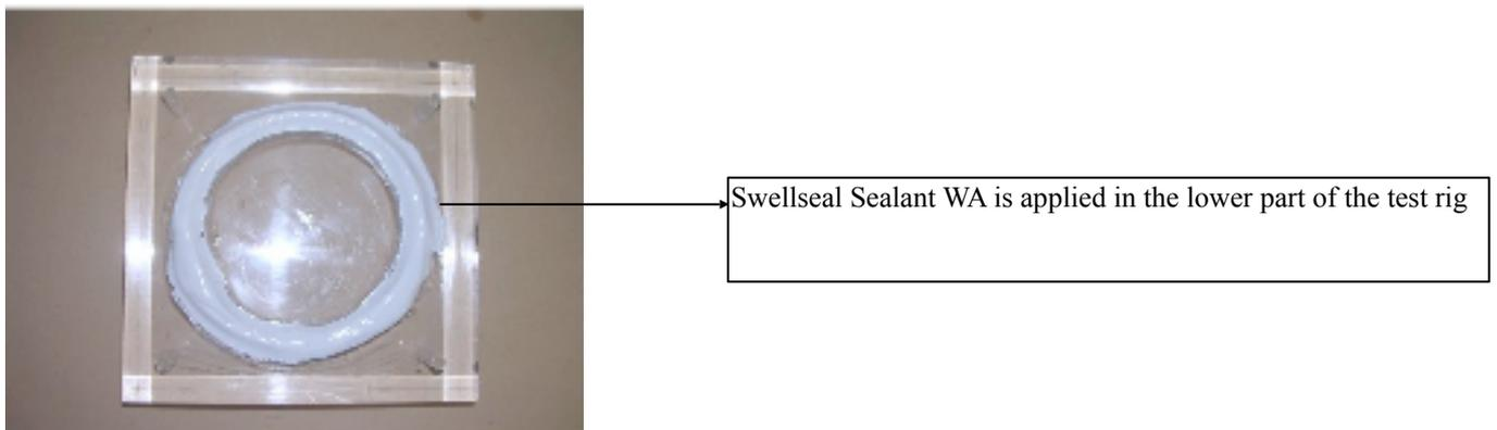
*Photo 2 : Swellseal Sealant WA after application in the joint*
