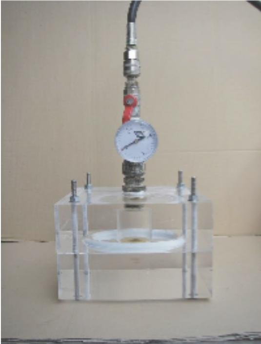
*Photo 5 : manometer indicating 10 bars after 10 days. No leaks detected.*
