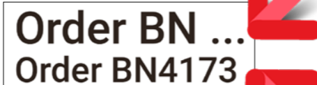
At runtime: At the top, with "ellipse": the content is truncated At the bottom, with "reduction": the font size has been automatically reduced, the entire content is displayed
