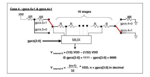
Fig.8: V<sub>internal R</sub> hardware connection if gpcs.5=1 and gpcs.4=1
