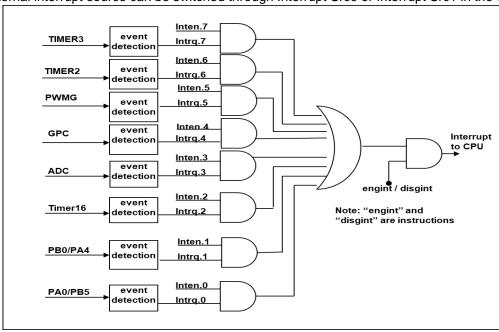
Fig.20: Hardware diagram of interrupt controller
