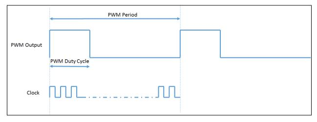
Fig.14: PWM Output Waveform
