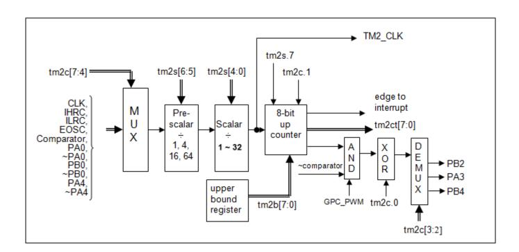
Fig.11: Timer2 hardware diagram
