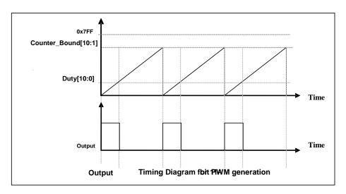
Fig.16: Output Timing Diagram of 11-bit PWM Generator
