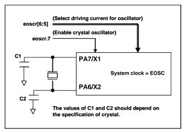
Fig.2: Connection of crystal oscillator
