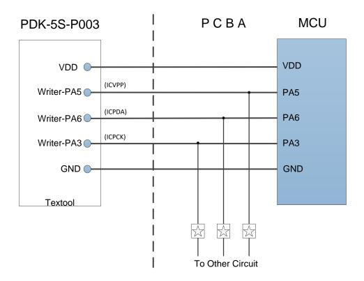
The above figure shows the connection for PFS123 on-board writing. In this figure,  $\frac{1}{2}$  can be either resistors or capacitors. They are used to isolate the programming signal wires from the peripheral circuit. it should be  $\geq 10$ K $\Omega$  for resistance while  $\leq 220$ pF for capacitance.
