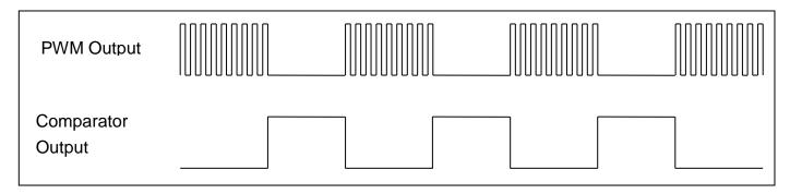
Fig.13: Comparator controls the output of PWM waveform
