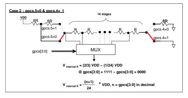
Fig.6: Vinternal R hardware connection if gpcs.5=0 and gpcs.4=1
