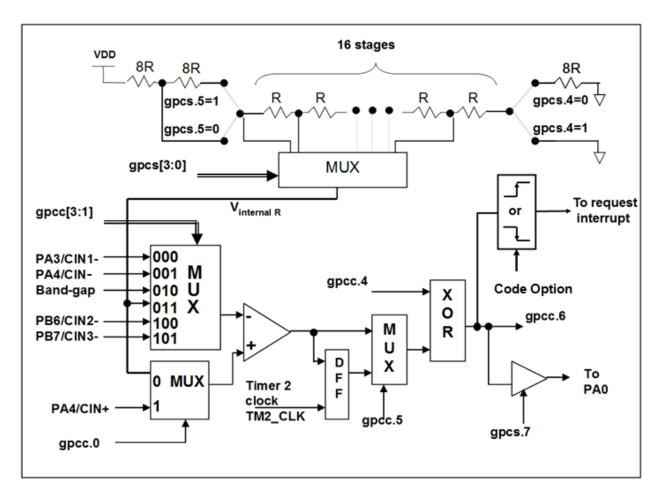
Fig.4: Hardware diagram of comparator
