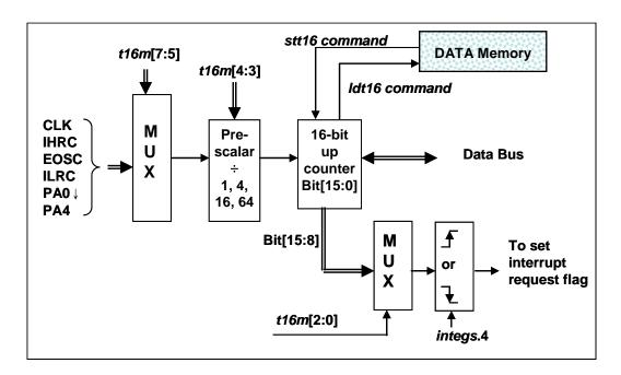
Fig.10: Hardware diagram of Timer16
