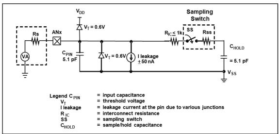
Fig. 23: Analog Input Model
