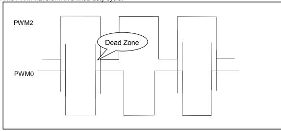
Fig.17: Complementary PWM waveform with dead zones
