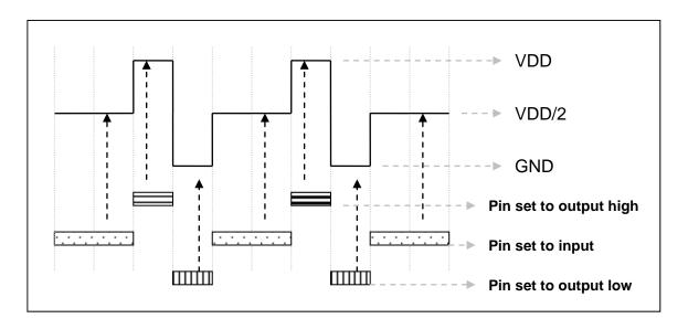
Fig. 9: Using VDD/2 LCD bias voltage generator
