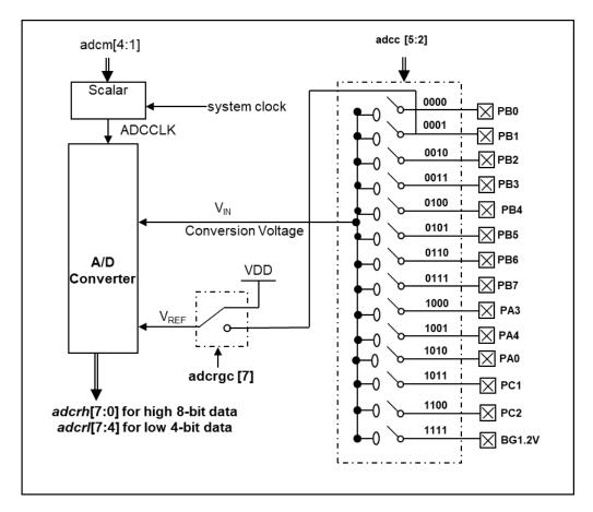
Fig. 22: ADC Block Diagram
