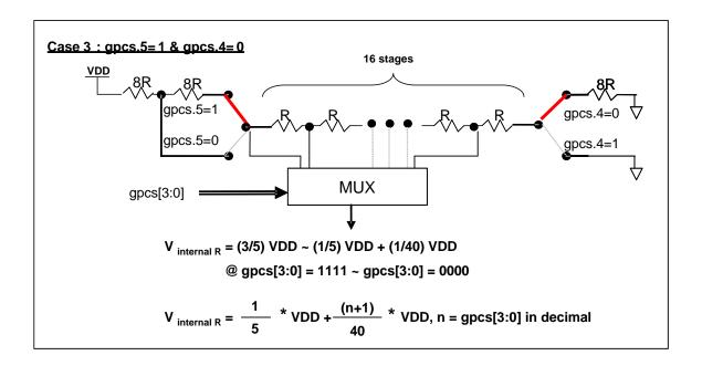
Fig.7: V<sub>internal R</sub> hardware connection if gpcs.5=1 and gpcs.4=0
