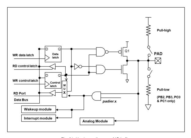
Fig. 21: Hardware diagram of IO buffer
