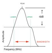
The relation between MHz bandwidth and waveform duration is shown in Figure (6). The scatter is wider at -40 dB because the 1% trailing end of the waveform contains very little energy and so has very little effect on the analysis of bandwidth. Because of the scatter it is most appropriate to specify waveforms in the time domain (microseconds) and spectra in the frequency domain.
