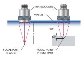
This change in the focal length can be predicted by Equation (13). For example, given a particular focal length and material path, this equation can be used to determine the appropriate water path to compensate for the focusing effect in the test material.
