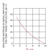
Increase In On-Axis Pulse-Echo Sensitivity Versus Normalized Focal Length
