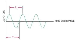
The number of cycles completed in one second is called frequency (f) and is measured in Hertz (Hz), with multiples as follows;
