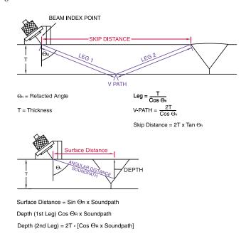
Many AWS inspections are performed using refracted shear waves. However, grainy materials such as austenitic stainless steel may require refracted longitudinal waves or other angle beam techniques for successful inspections.
