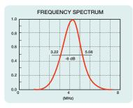
Signal waveform and frequency spectrum of DL4R-3.5X10
