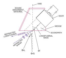
The incident angle necessary to produce a desired refracted wave (i.e. a  $45^{\circ}$  shear wave in steel) can be calculated from Snell's Law as shown in Equation (12). Because of the effects of beam spread, this equation doesn't hold at low frequency and small active element size. Contact us for details concerning these phenomena.
