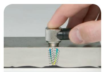
Two angled elements create a V-shaped sound path in the test material. This pseudo-focus enhances resolution in the focal zone.
