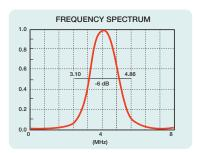
Signal waveform and frequency spectrum of AM4R-8X9-45  $\,$
