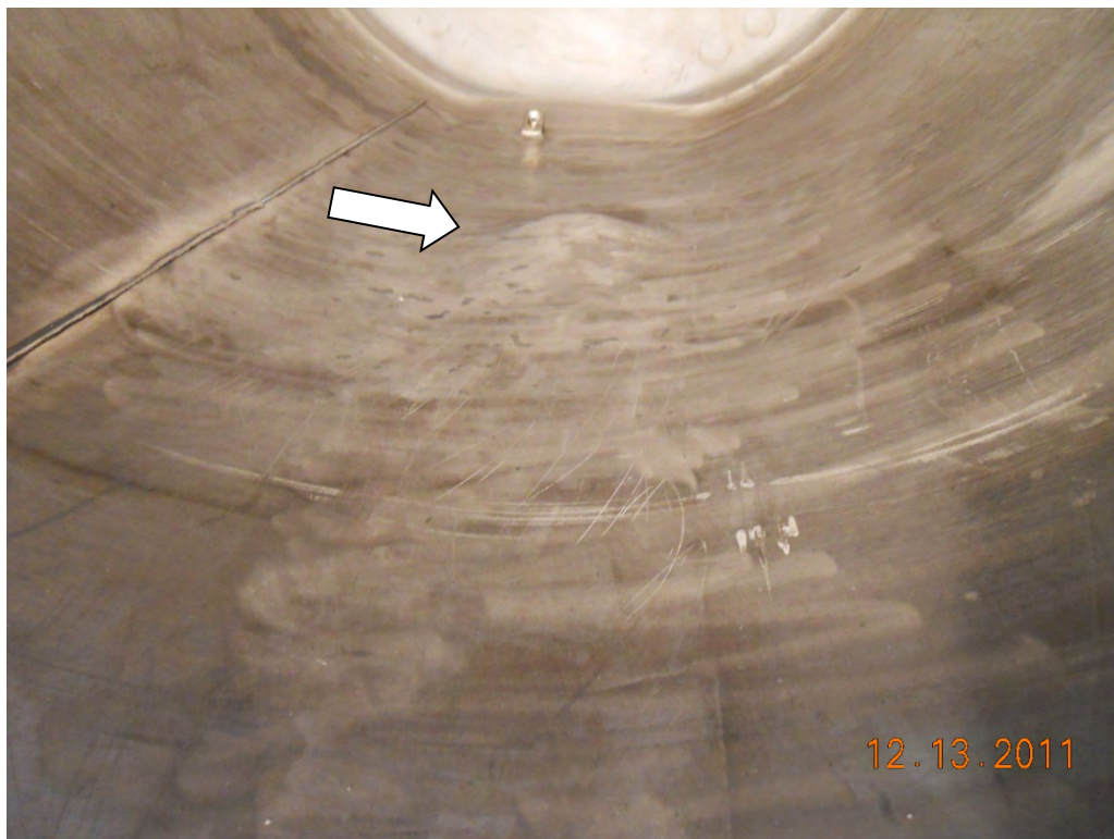
Figure 2.12.3-35 – Internal View of Damage from Puncture Test P7
