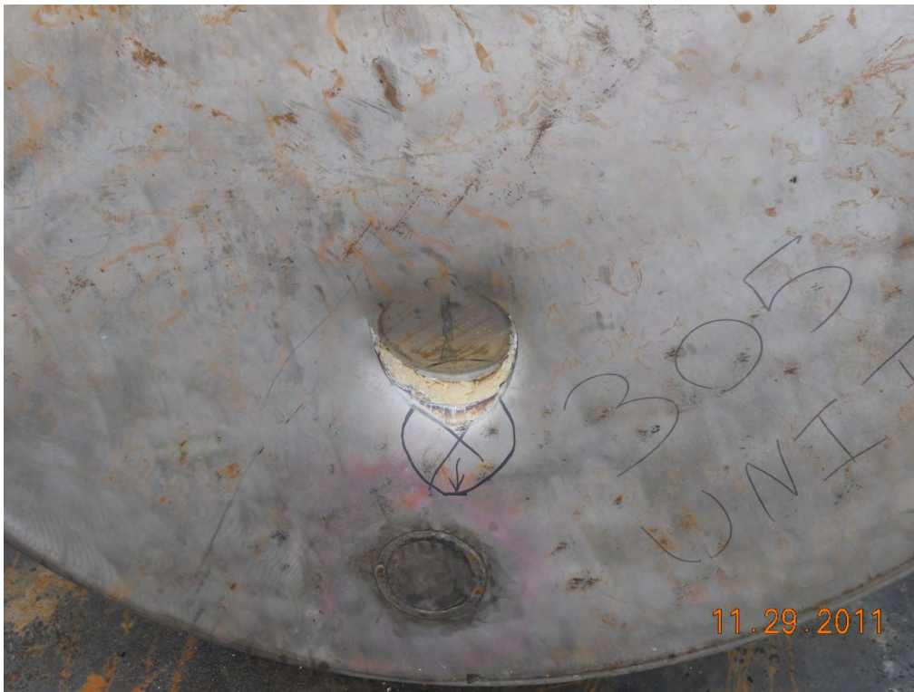
Figure 2.12.3-7 – Damage to Impact Limiter Bottom Due to Puncture Drop Test P1
