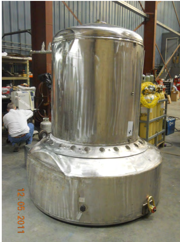
Figure 2.12.3-17 – CTU #1 Condition After Free Drop Test D2H
