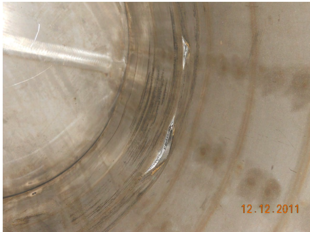
Figure 2.12.3-37 – Cut in Inner Container (IC) Wall Due to Dummy Payload Side Impact
