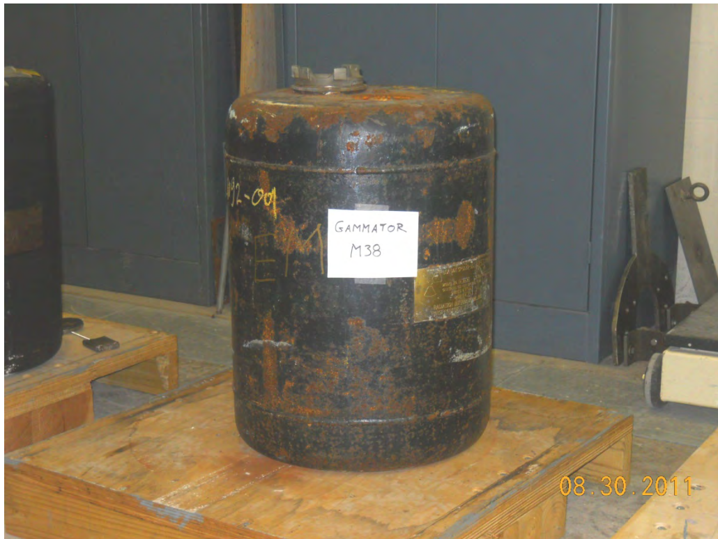
Figure 1.2-13 – Gammator M38 Shielded Device
