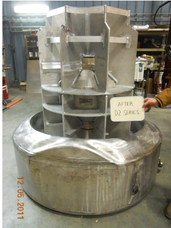
Figure 2.12.3-20 – General Condition of Lodgment & LTSS After D1 and D2 Test Series
