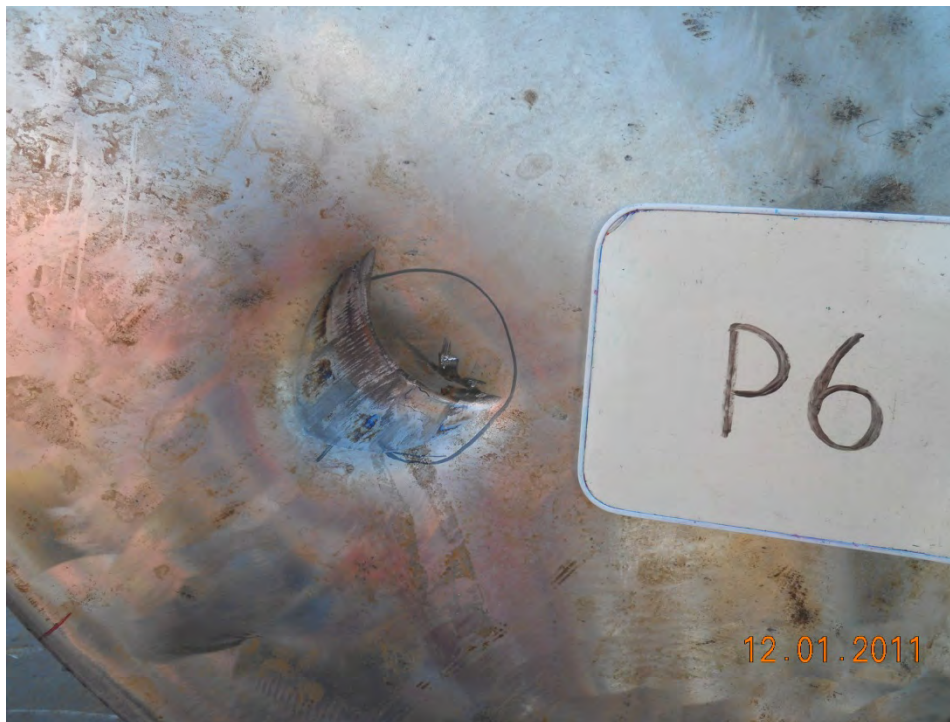
Figure 2.12.3-13 – Damage to Impact Limiter Bottom Due to Puncture Drop Test P6
