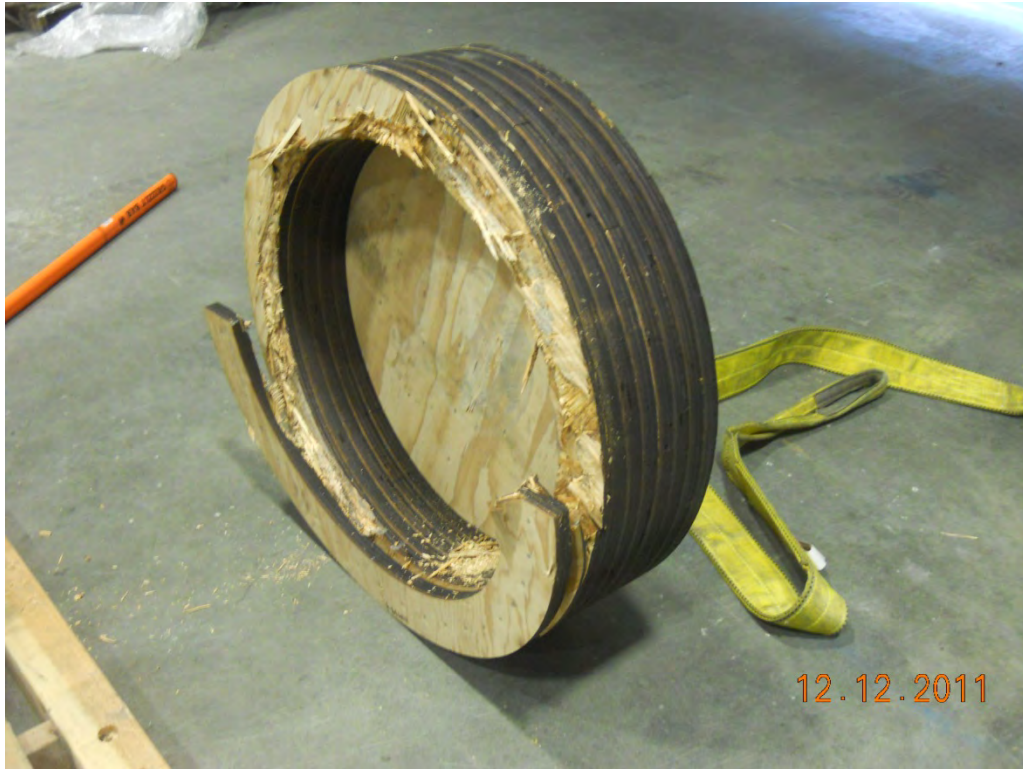
Figure 2.12.3-38 – Dunnage After D6 Test Series
