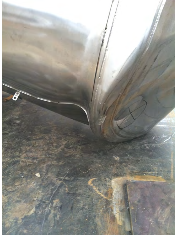
Figure 2.12.3-26 – Detail of Puncture Test P3 Damage
