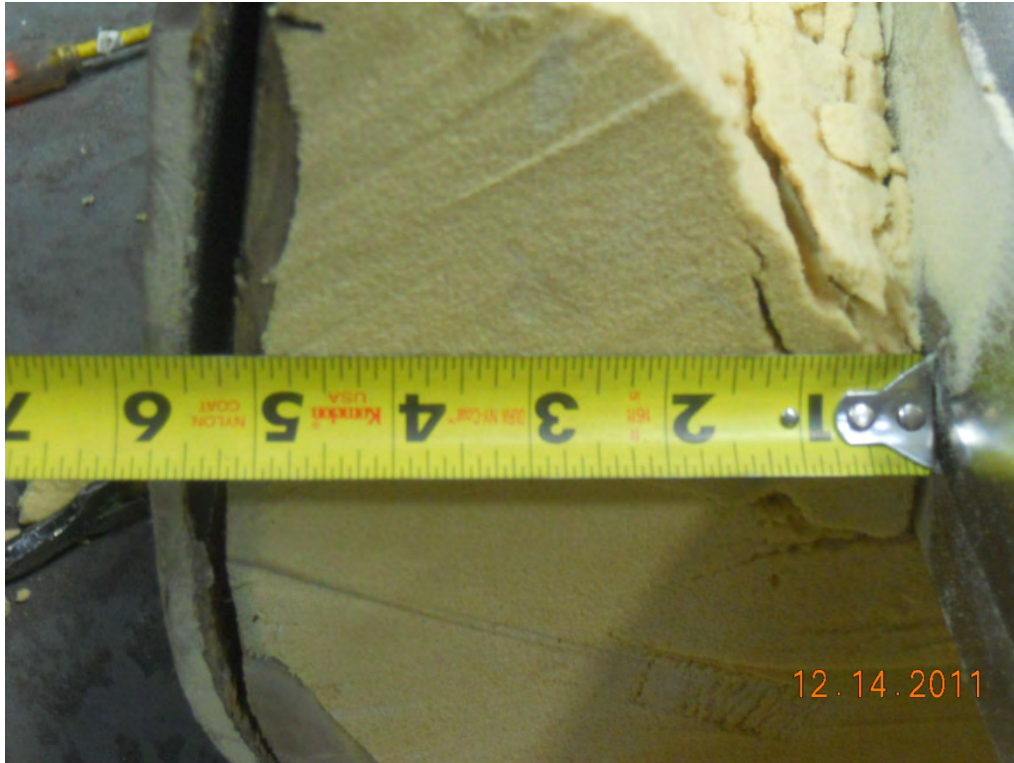
Figure 2.12.3-48 – Minimum Foam Remaining After Free Drop D4H
