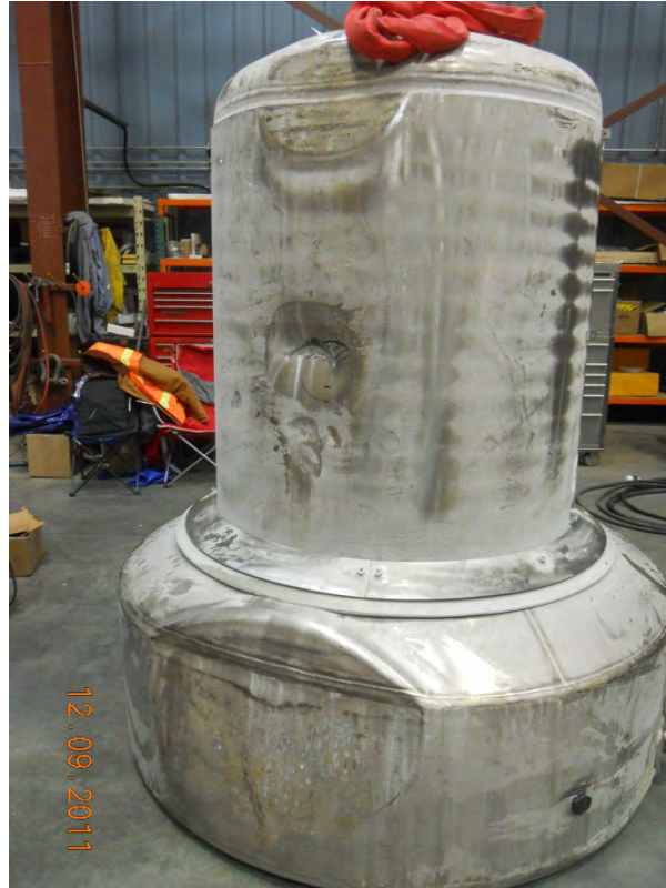
Figure 2.12.3-28 – CTU #3 Condition After Free Drop Test D6H (Also Showing P7)
