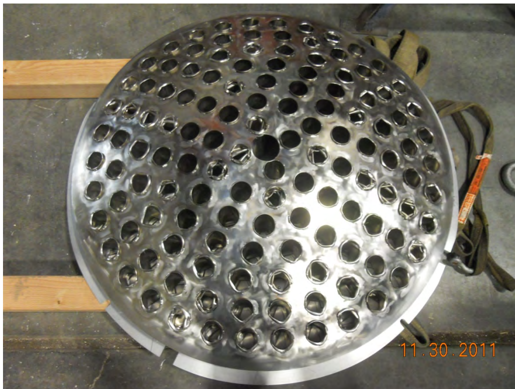
Figure 2.12.3-9 – Lower internal impact limiter, View From Beneath, After D1 Test Series
