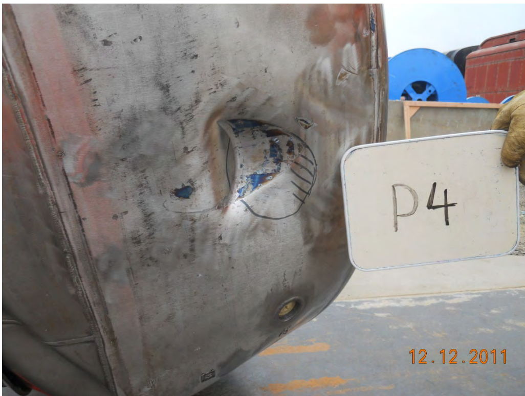
Figure 2.12.3-43 – Damage to Impact Limiter Side Due to Puncture Drop Test P4
