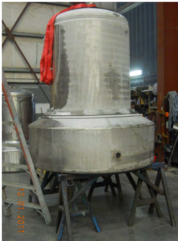
Figure 2.12.3-11 – CTU #3 Condition After Free Drop Test D5H
