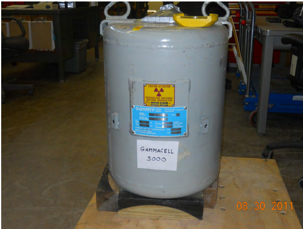
Figure 1.2-15 – Gammacell 3000 Shielded Device
