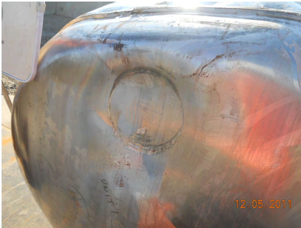
Figure 2.12.3-19 – Damage to Package Top Due to Puncture Drop Test P2
