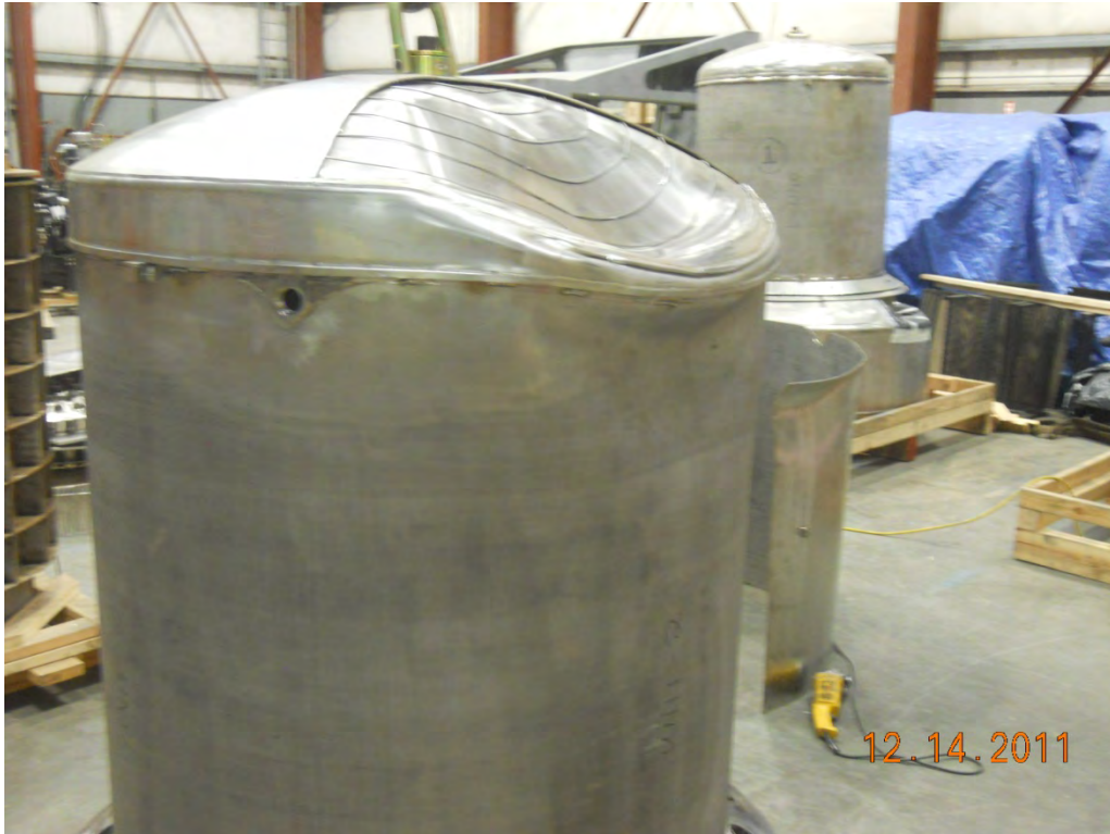
Figure 2.12.3-46 – View of Damage Due to Test Series D3
