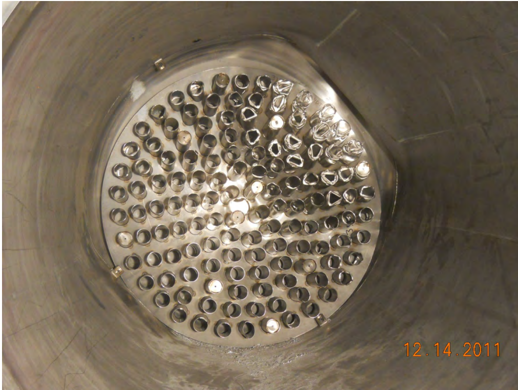
Figure 2.12.3-44 – Crushed Internal impact limiter Tubes (Upper) Due to Free Drop D3
