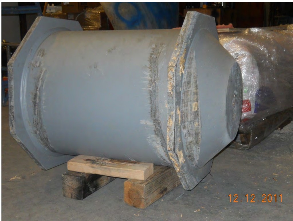
Figure 2.12.3-39 – Dummy Payload After D6 Test Series
