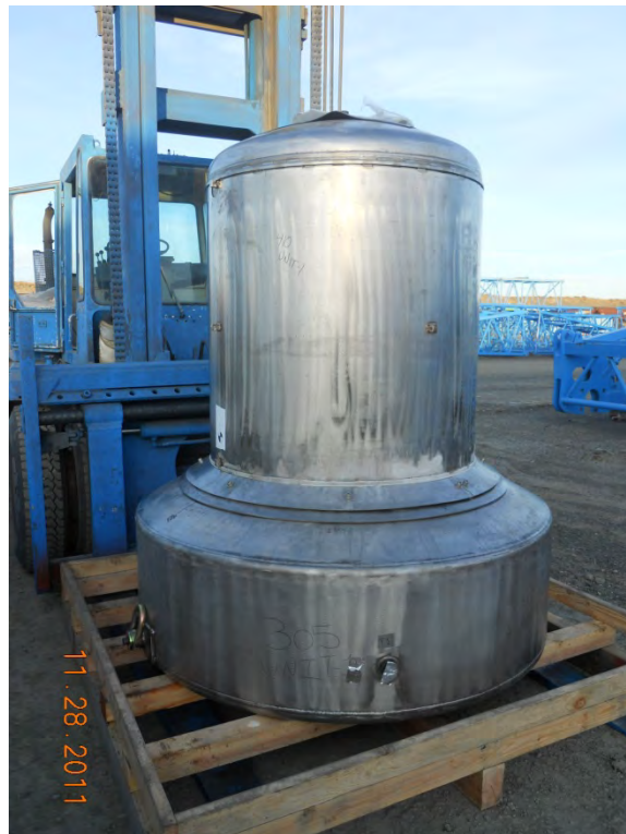
Figure 2.12.3-5 – CTU #1 Condition After Free Drop Test D1H
