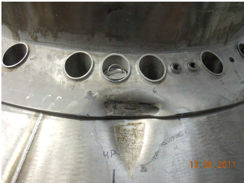
Figure 2.12.3-33 – Detail of Puncture Test P5 Damage (Rain Shield Removed)
