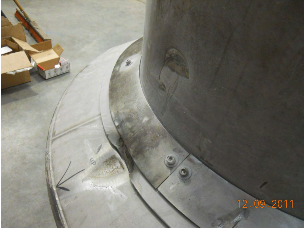
Figure 2.12.3-32 – Damage to Package Side Due to Puncture Drop Test P5
