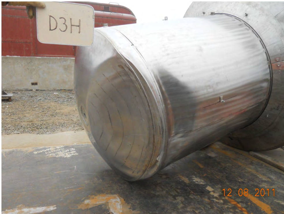
Figure 2.12.3-23 – CTU #2 Condition After Free Drop Test D3H
