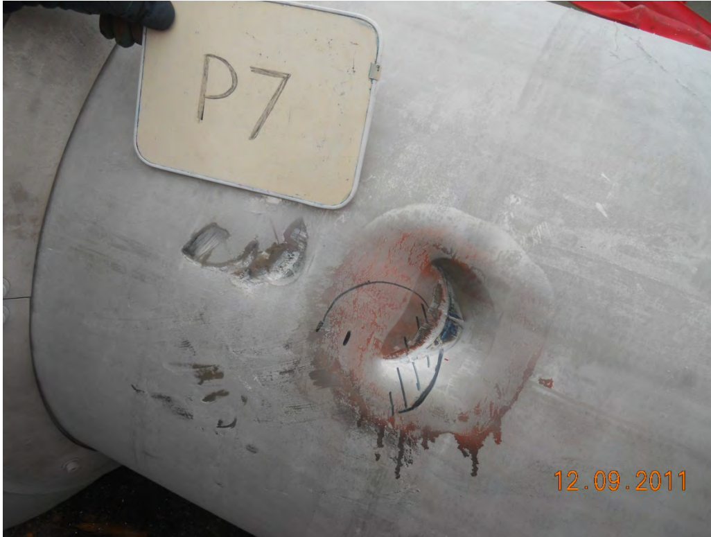
Figure 2.12.3-30 – Damage to Package Side Due to Puncture Drop Test P7
