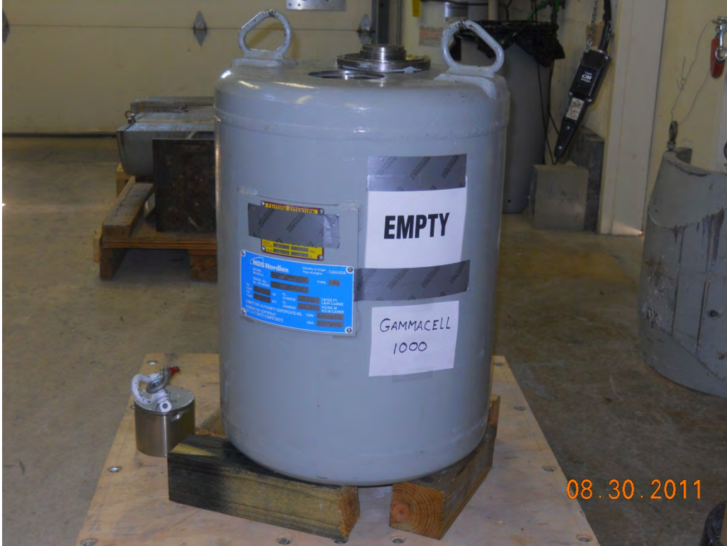
Figure 1.2-14 – Gammacell 1000 Shielded Device
