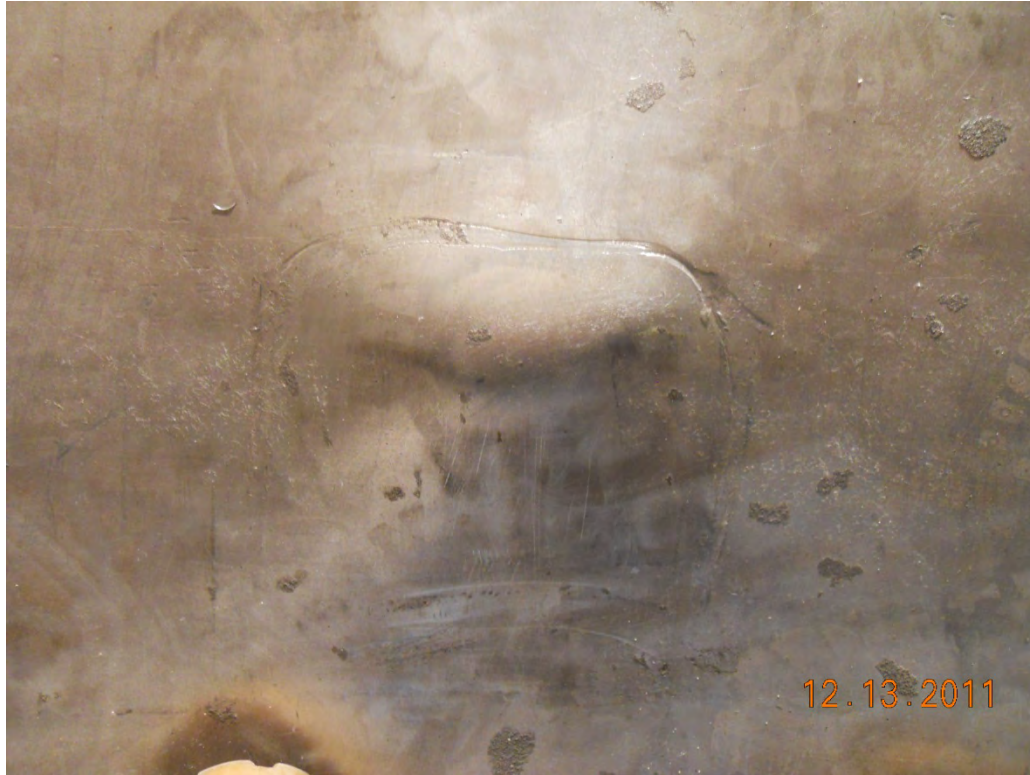
Figure 2.12.3-36 – Internal View of Damage from Puncture Test P7, Detail
