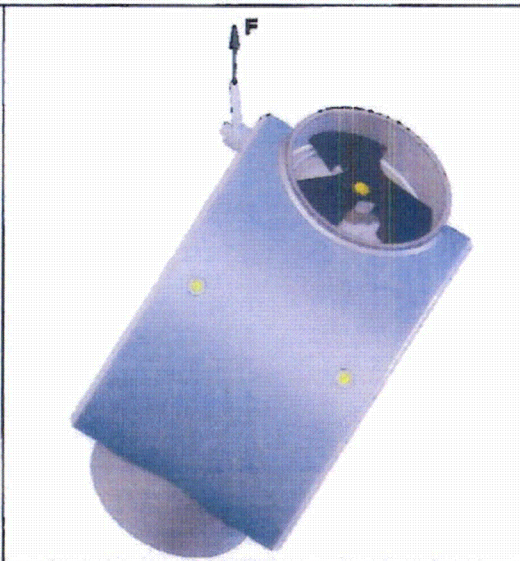
Figure 11 SENTRY Lifted by a Single Rivnut -Side View
