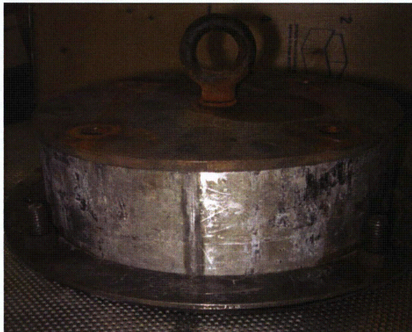
Figure 4-2 – PCI Stacked Disk Strainer with Support Ring (Top Plate Bolts Not Shown)
