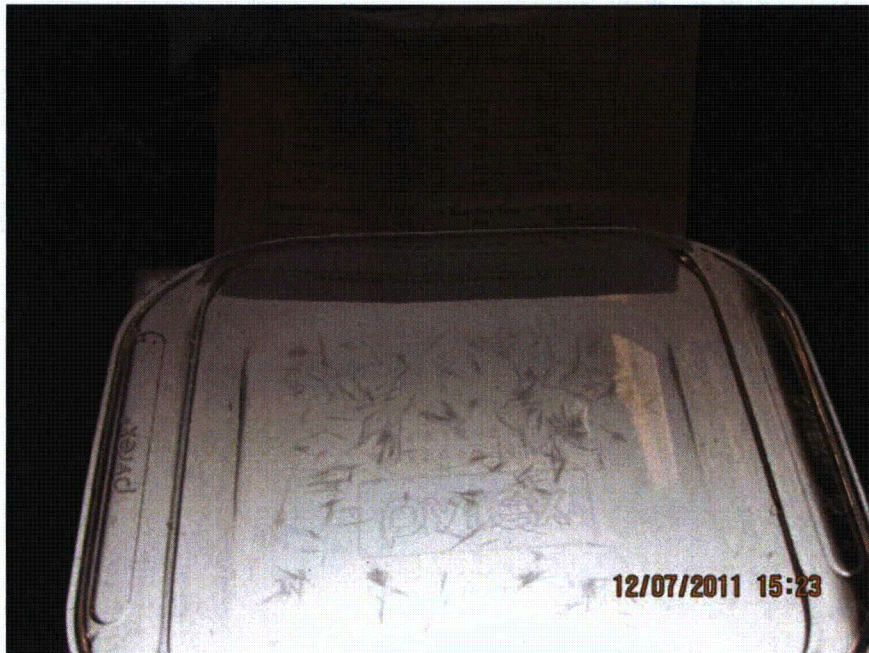
Figure 4-6 – Prepared Bypass Test Temp-mat Fines
