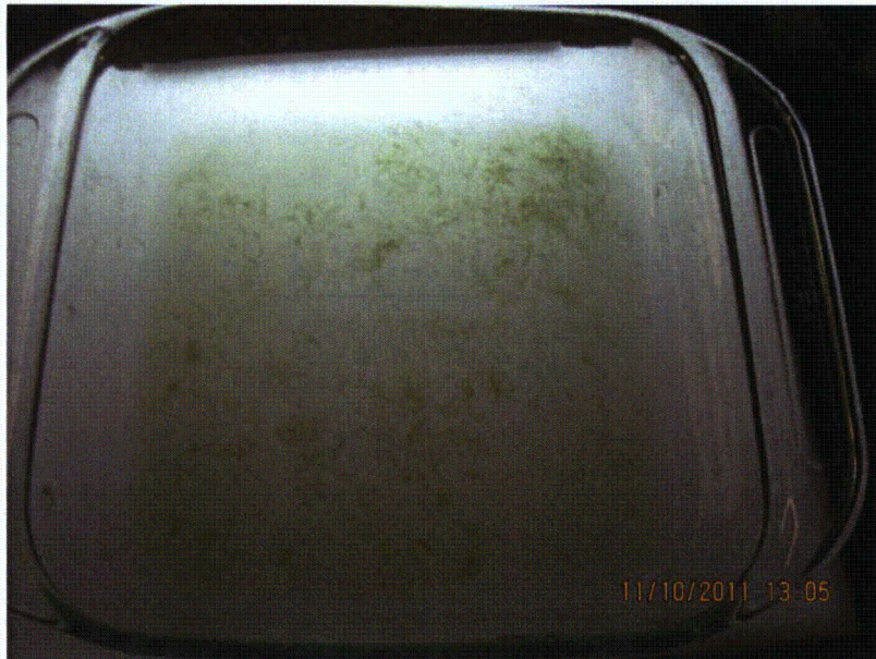
Figure 4-4 – Prepared Bypass Test NUKON Fines
