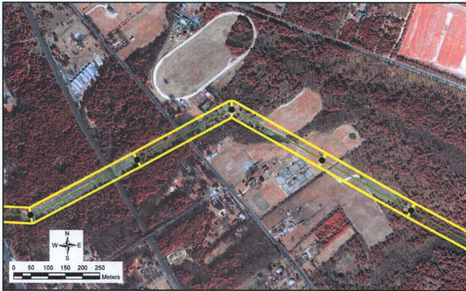
Figure 1.2. An example of a single ROW corridor with individual spans in yellow, the circuit path in green, and tower locations as black dots on a 2002 aerial photograph.
