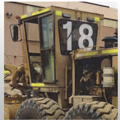
Equipment ID Decals
