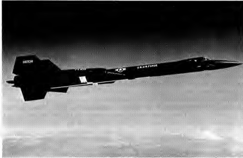
December 11: USAF YF-12A supersonic aircraft made its first research flight from Edwards AFB, to open a joint NASA-USAF program to advance knowledge of high-performance flight. Special instrumentation installed by NASA increased the value of the flying test bed for accumulating data. Pilots were from NASA and the Air Force.
