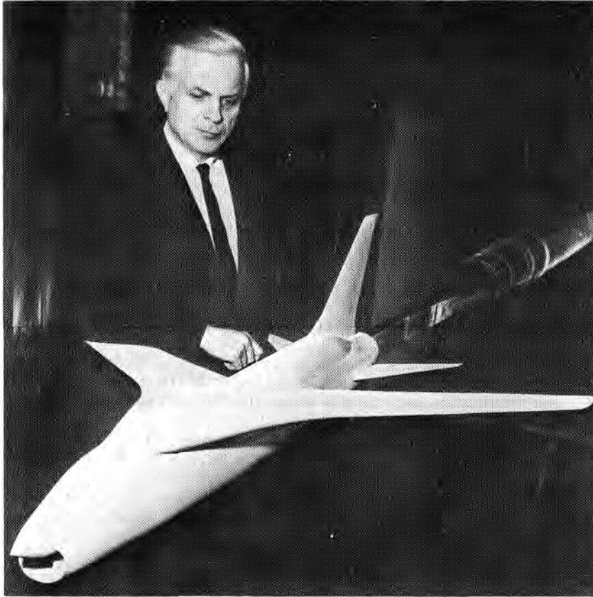
February 9: NASA announced the supercritical wing, a new airfoil shape developed in four years of wind-tunnel studies at Langley Research Center, would be flight-tested on a USN F-8 fighter at the Flight Research Center. Dr. Richard T. Whitcomb, inventor of the design expected to improve performance of subsonic jet transports, stood with his model in the test section of the wind tunnel at LARC.
