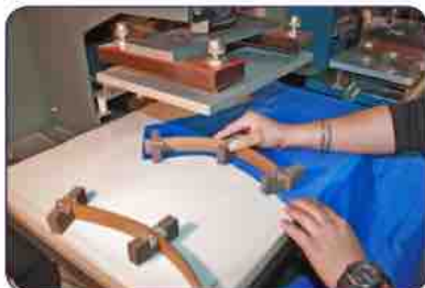
Custom fitting the RF sealing welds.
