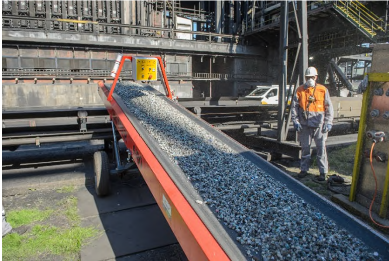
Figure 97: SRF pellet feeding during industrial tests in the coking plant
