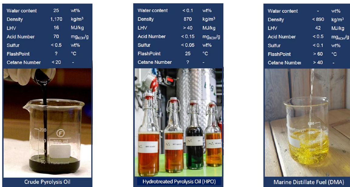
Figure 11: Change in composition of pyrolysis oil (left) when it is converted to HPO (middle), which is comparable to fossil DMA (right).
