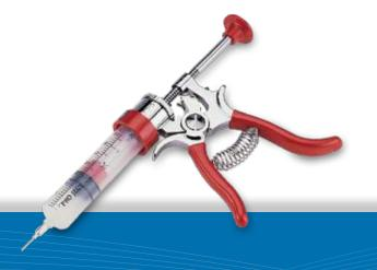
The AD93 volumetrically dispenses epoxies, silicones, glues and pastes. Available in two capacities, 35cc and 80cc syringe, with hot stamped sidewall indicators for dosage levels in cc and ounces. Shot sizes can be selected in increments of 1cc to 5cc. Material delivery is via luer lock tips.
