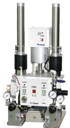
The EP1320C tandem cartridge pump is designed to easily transfer material for controlled dispensing via a high pressure valve. The suitable viscosity range is 10,000cps - 600,000cps. Rated at 15:1 the system provides a maximum of 995 psi regulated material pressure. The A & B cartridge management automatically switches from either A to B or B to A when the cartridge is exhausted. Cartridges are contained in metal jacketed cylinders.
