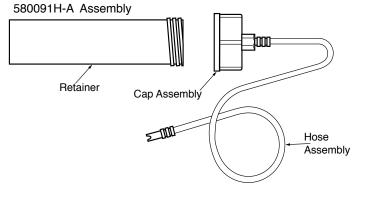
Dispense caulk and sealant materials. Connect the 580112C to a regulated air supply to dispense directly from the caulking tube. Most materials will dispense satisfactorily from 12 to 30 psi (0.80 - 2.0bar). Do not exceed 60 psi (4 bar).
