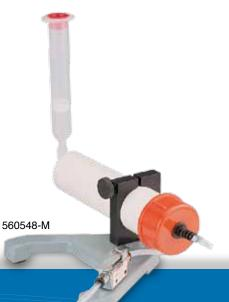
The model 560548-M loads a barrel directly from a 1/10 gallon caulking tube. The model 560022-M loads a barrel from a 12 ounce cartridge. The barrel loader is connected to an air regulator and set to a pressure suitable for the material but less than 65psi (4.48 bar). A switch on the side of the stand activates the airflow and is switched off when the material reaches the desired level. The barrel attachment assembly is threaded to accept luer lock barrels.
