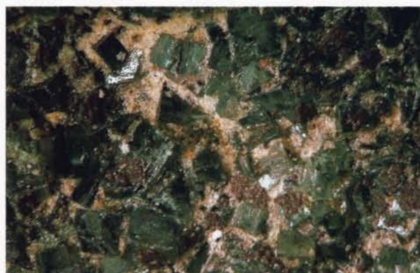
Figure 3. Dark green cubic crystals of bariopharmacosiderite up to 1 mm on edge collected from loose scree on the east side of the valley. Tony Rigby Collection.
