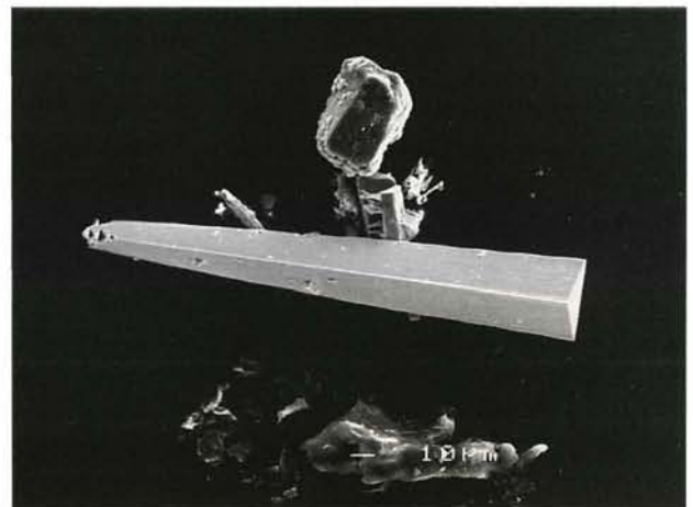
Figure 47. SEM photograph illustrating an unusual crystal habit of susannite, a trigonal prism growing from a point and gradually increasing in size along its length to a pinacoid termination.
