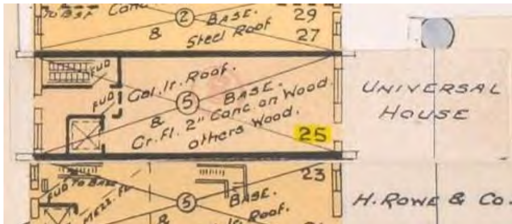
Figure 7. Section taken from a 1948 Mahlstedt plan shows interior alterations including the repositioning of the lift and stairwell and the closing up of interior openings between no 25 and 27-29 Elizabeth Street. (Source: Mahlsted Map, no 15, 1948)
