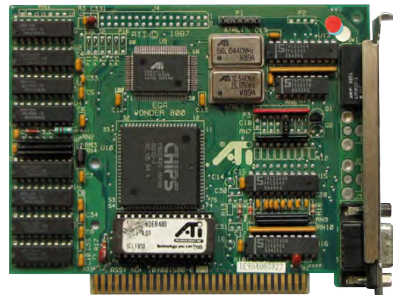
Using Chips and Technologies' EGA chipset, early graphics card manufacturers such as ATI could produce smaller, cheaper boards. Credit: Vlask, CC BY-SA 3.0
