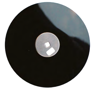
Inside a 3.5in disk's plastic shell is a small floppy disk with a piece of protective fabric on either side
