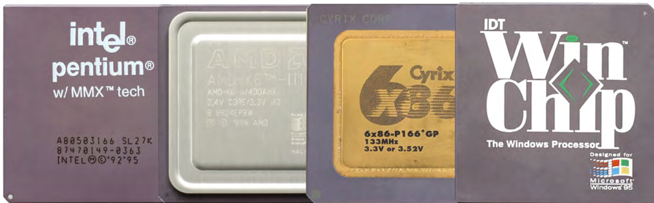
Socket 7 supported CPUs from multiple manufacturers, including Intel, AMD, Cyrix and IDT. Photo credit: Konstantin Lanzet
