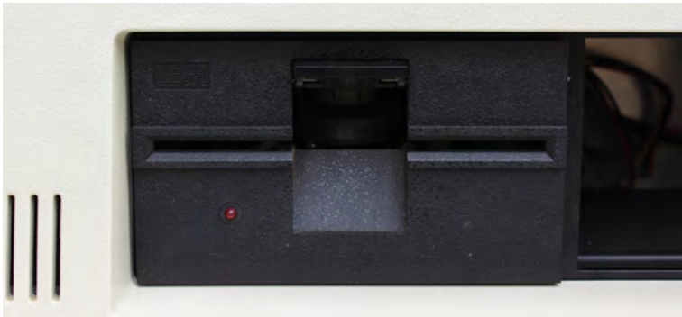
A 5.25in floppy drive was the standard storage system for the 5150, with no hard drive option at launch
