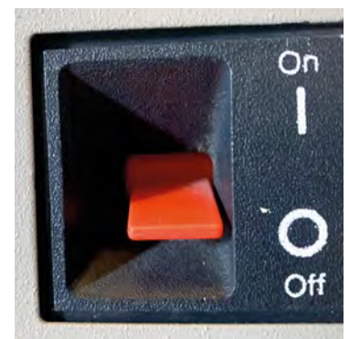
You flip the big red switch (BRS) on the side to power the PC 5150 up or down
