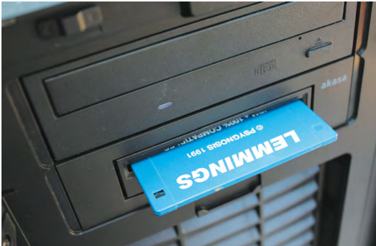
An Akasa 3.5-to-5.25in bay adaptor enables us to fit a floppy drive in our Fractal Design Define R5. Yay, Lemmings!
