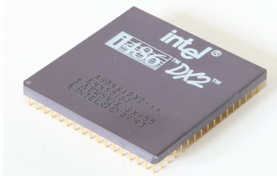
The 2nd-generation DX2 chips doubled their predecessors' clock speed, a feat never replicated by any subsequent Intel CPU. Image credit: Henry Mühlfordt, own work, CC BY-SA 3.0
