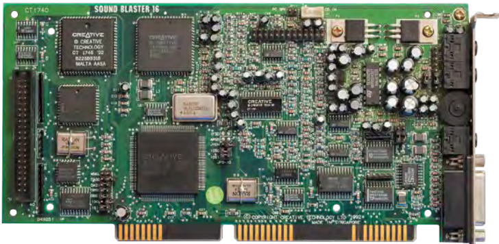
Creative's Sound Blaster 16 will happily provide FM synthesiser music in games, as well as sampled sound
