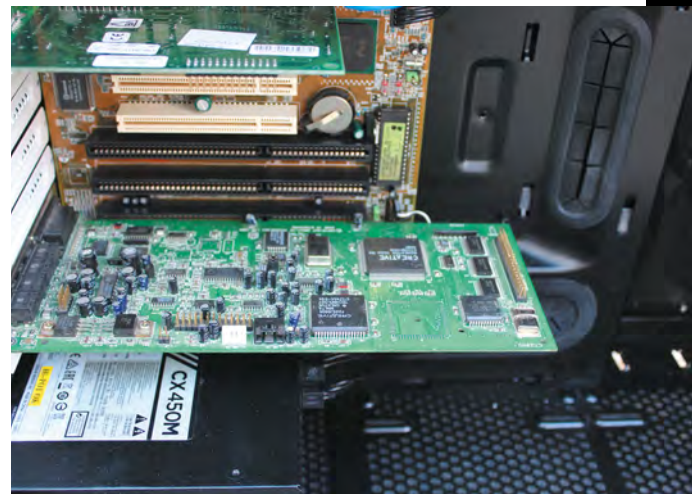
ISA cards have the PCB on the other side of the backplate from PCI cards
