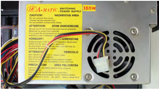
The floppy drive connects to a 4-pin Molex connector on the PSU – a plug that’s still sometimes used in today’s PCs
