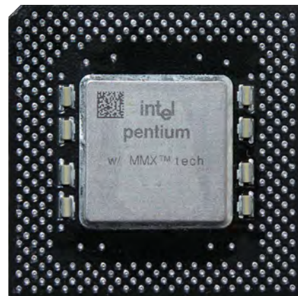
We're using a 166MHz Intel Pentium MMX CPU
