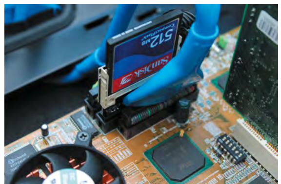
Our CompactFlash adaptor, CD-ROM and floppy drive are all connected to the right sockets, with power and rounded cables routed via the cable-routing holes
