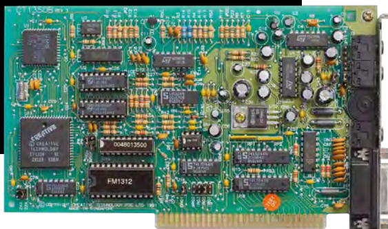
The later Sound Blaster 2 increased the playback sampling rate to 44KHz, still on an 8-bit ISA card
