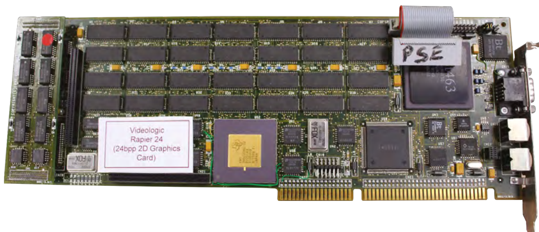
An early ISA Rapier 24 card – the big gold Texas Instruments chip handles transform and lighting
