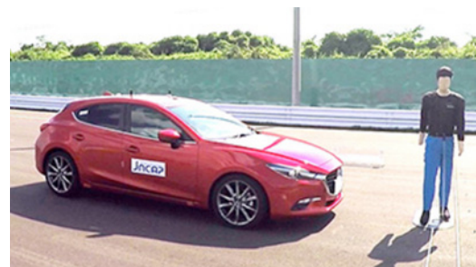
Testing automatic brake for pedestrians (Photo by: NASVA)
