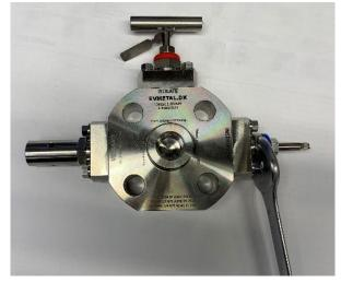
3. Tighten the stem sealing by turning the gland clock wise using a 13 mm key. Note, use a closed key to avoid damaging the hexagon.
