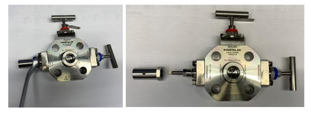
2. Tighten the stem sealing by turning the gland clock wise using a 13 mm key. Note, use a closed key to avoid damaging the hexagon.
