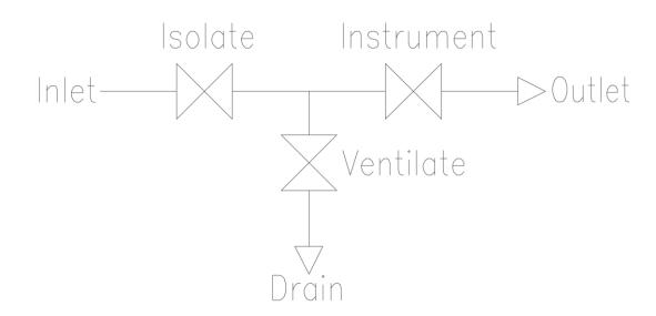
Isolate and Ventilate is normally operated with a T-handle. Isolate valve is marked with red dust cap. The Instrument valve is marked with blue dust cap. The ventilate valve must be operated with a 5 mm square key.
