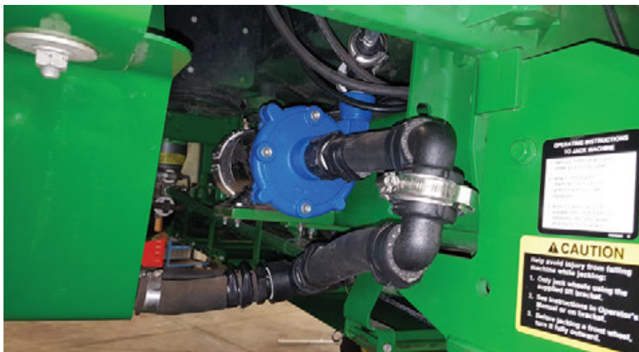
Figure 2. An electric pump dedicated to the clean water tank helps with rinsing the sprayer plumbing.
