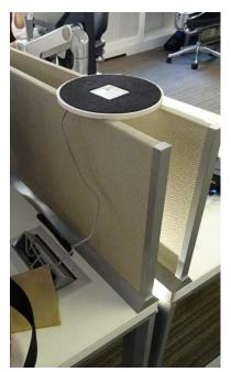
*Figure 5. A sensor-controlled task light annoyed one occupant who turned it upsidedown, rather than simply turning it off.*
