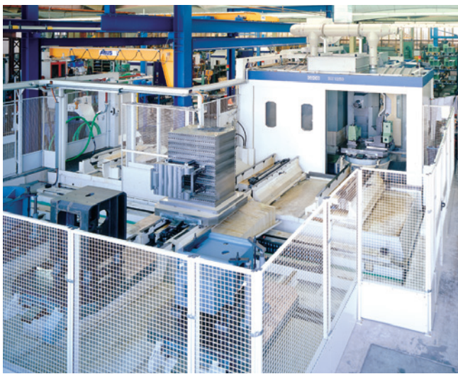
Flexible production cell with pallet changer station. In our production we are using machining centres from ALZMETALL, GROB, HELLER and STARRAG-HECKERT.
