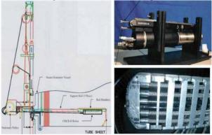
Fig. 1. Lancing Equipment Used for Hanul Unit 2
