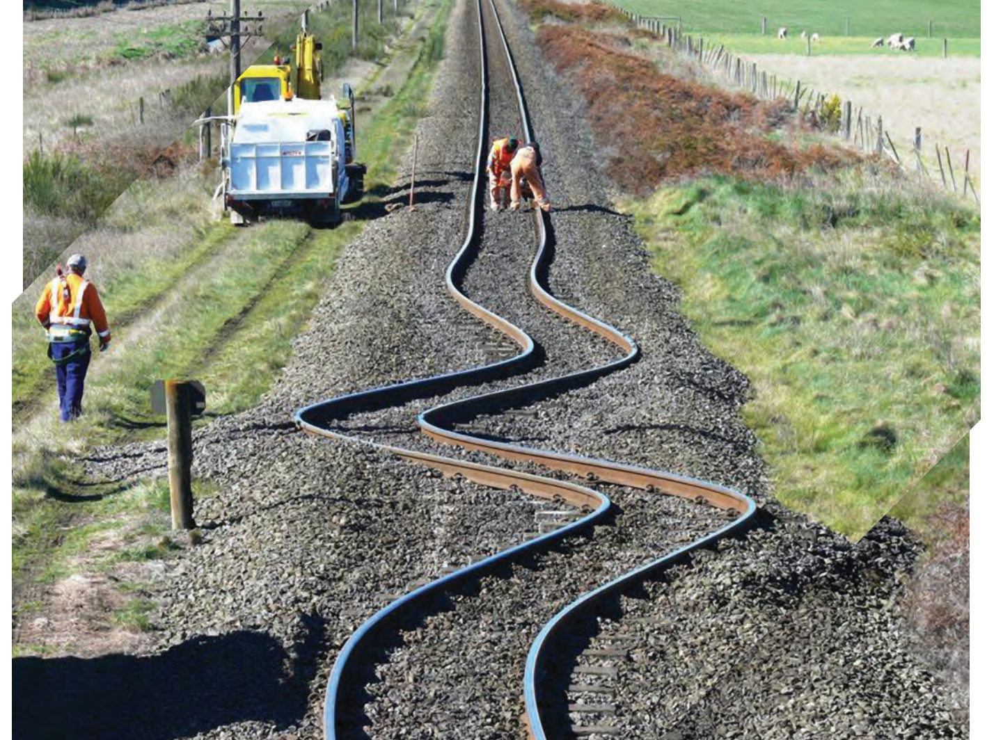
Railroad tracks bent by the 2010 Canterbury earthquake. The tracks crossed the fault rupture near Rolleston, New Zealand.
