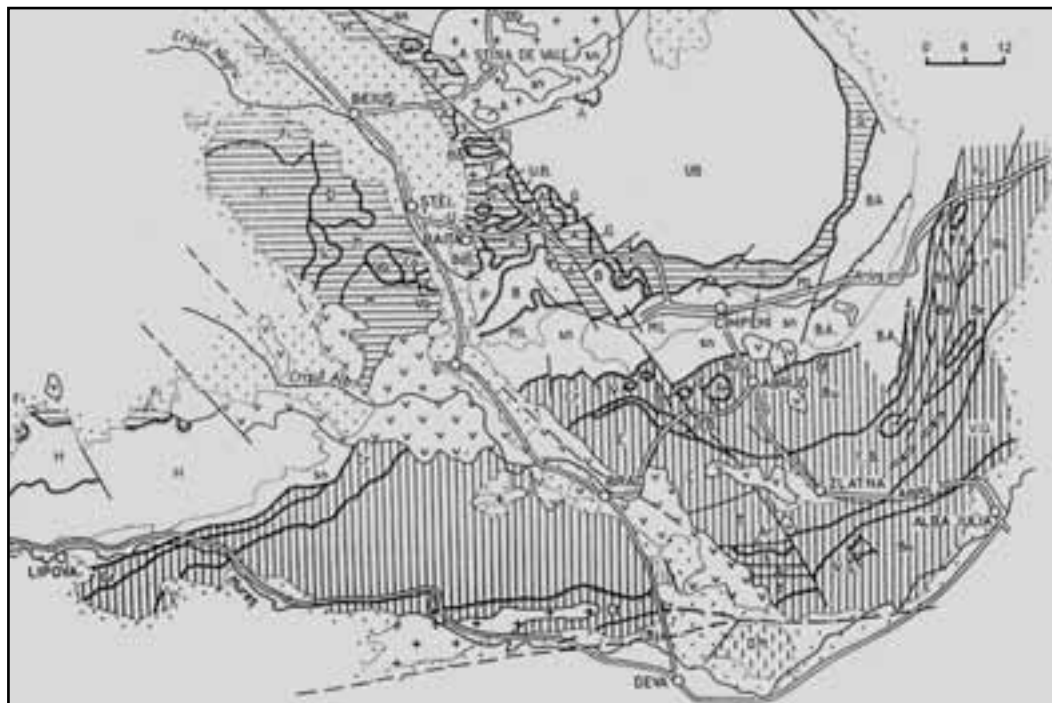
Figure 7 - Structural sketch-map of the Apuseni Mountains. .... Neogene molasse cover; vvvv Neogene calc-alkaline magmatites; +++ Upper Cretaceous calc-alkaline magmatites; Sn, post-tectogenetic cover of the North Apusenides. Northern Apusenides: Biharia Nappes System – BA, Baia de Arieș Nappe; ML, Muncel-Lupșa Nappe; B, Biharia Nappe; H P, Highiș (H) and Poiana (P) Nappes; Codru Nappes System: Co, Colești Nappe; Va, Vașcău Nappe; M A, Moma (M) and Arieșeni (A) Nappes; Vt, Vetre Nappe; D Ba, Dieva (D) and Bătrânescu (Ba) Nappes; S F, Șasa (S) and Ferice (F) Nappes; U, Următ Nappe; Fi G, Finiș (Fi) and Gârda (G) Nappes; Vl, Vălani Nappe; UB, Bihor Unit. Southern Apusenides: Ri, Rimetea Nappe; Be, Bedeleu Nappe. Bedeleu Nappes System: Fu, Fundoia Nappe; H, Hospea Nappe; Bj, Bejani Unit; Bo, Bozeș Nappe; V Ar, Vulcan (V) and Ardeu (Ar) Nappes; Cb, Căbești Nappe; VG, Valea Mică-Galda Nappe; T, Techerău Nappe; C, Curechiu Nappe; FB, Feneș-Blăjani Nappe; Cr Fr, Criș (Cr) and Frasin (Fr) Nappes; Gr, Groși Nappe; Bu, Bucium Unit. Median Dacides: DM, Supragetic Nappes
